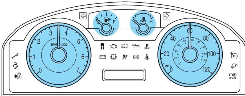
**Speedometer:** Indicates the current vehicle speed.
