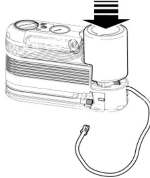
3. Wrap the clear tube around the compressor housing.
