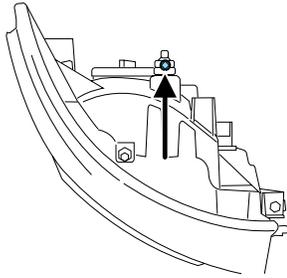
5. Locate the vertical adjuster on each headlamp. Using a Phillips #2 screwdriver, turn the adjuster either clockwise (to adjust down) or counterclockwise (to adjust up). The horizontal edge of the brighter light should touch the horizontal reference line.
