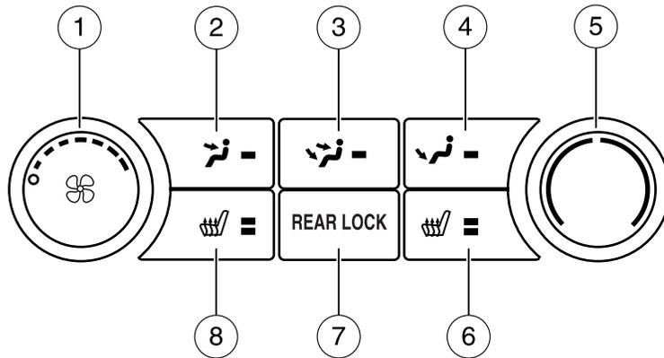
1. **Fan speed:** Turn to select the desired fan speed.
