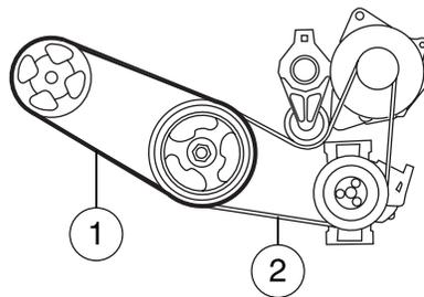
1. Short drivebelt is on first pulley groove closest to engine.
