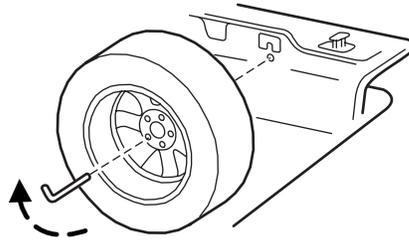
**If you are stowing the temporary spare tire,** place the tire over the jack and secure it with the large wing nut.
