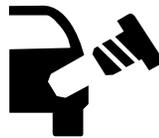
**Brake system warning light:** To confirm the brake system warning light is functional, it will momentarily illuminate when the ignition is turned to the on position when the engine is not running, or in a position between on and start, or by applying the parking brake when the ignition is turned to the on position. If the brake system warning light does not illuminate at this time, seek service immediately from your authorized dealer. Illumination
