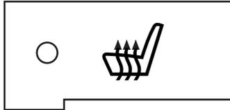
The heated seats will activate when the ignition is in the on position and the engine is running.
