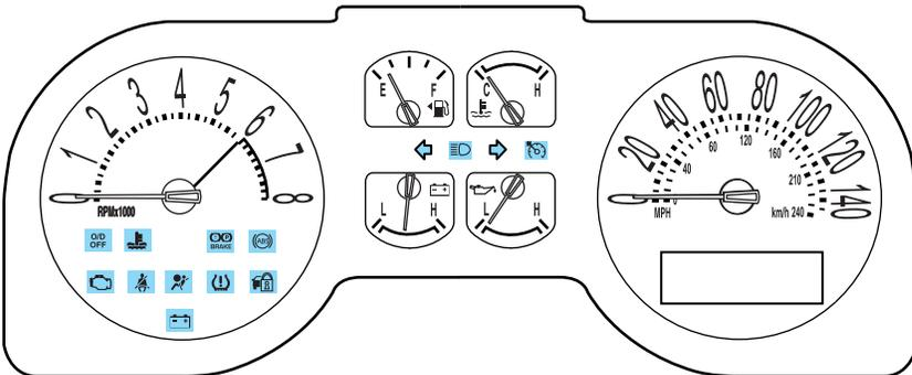
Warning lights and gauges can alert you to a vehicle condition that may become serious enough to cause extensive repairs. A warning light may illuminate when a problem exists with one of your vehicle's functions. Many lights will illuminate when you start your vehicle to make sure the bulbs work. If any light remains on after starting the vehicle, refer to the respective system warning light for additional information.
