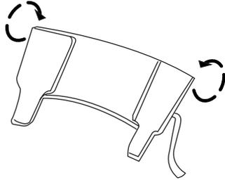
1. Position the boot right-side up and fold each side of the boot inward.
