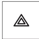
Push in the flasher control and all front and rear direction signals will flash. Press the flasher control again to turn them off. Use it when your vehicle is disabled and is creating a safety hazard for other motorists.
