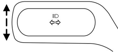
The flash rate of the turn signal indicator will speed up considerably if the Lighting Control Module detects a left or right turn lamp bulb (front or rear) is burned out.
