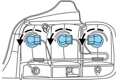
4. Disconnect the electrical grommet by pulling it straight off of the lamp assembly.
