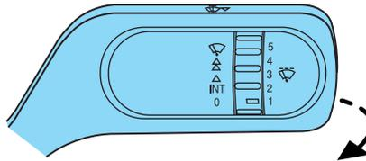
**Courtesy wipe feature:** One extra wipe will occur a few seconds after washing the front window to clear any excess washer fluid remaining on the windshield.
