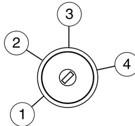
**Note:** If the engine does not start within five seconds on the first try, turn the key to off, wait 10 seconds and try again. If the engine still fails to start, press and hold the accelerator to the floor and try again; this will allow the engine to crank with the fuel shut off in case the engine is flooded with fuel.
