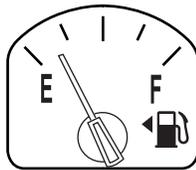
The FUEL icon and arrow indicates which side of the vehicle the fuel filler door is located.
