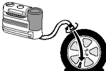
**Note:** When the sealing compound is first added into the tire, the air pressure gauge reading on the compressor unit may indicate a higher value; this is normal and should be no reason for concern. The pressure will drop after about 30 seconds of operation. The tire pressure has to be checked with the compressor in the OFF position to get the correct tire pressure reading.
