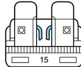
**Note:** Always replace a fuse with one that has the specified amperage rating. Using a fuse with a higher amperage rating can cause severe wire damage and could start a fire.
