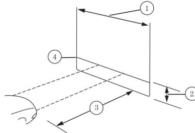
2. Measure the height from the center of your headlamp to the ground and mark an 8 foot (2.4 meter) horizontal reference line on the vertical wall or screen at this height (a piece of masking tape works well). The center of the lamp is marked by a 3.0 mm circle on the headlamp lens.
