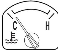
If the engine reaches a preset over-temperature condition, the engine will automatically switch to alternating cylinder operation. Each disabled cylinder acts as an air pump and cools the engine.
