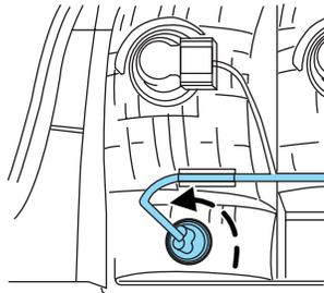
4. Remove the three nut and washer assemblies and the lamp assembly from the vehicle.
