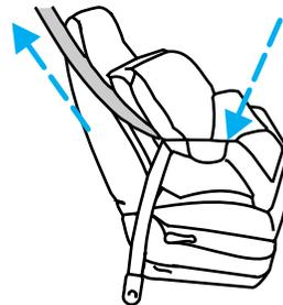
9. Attach the tether strap (if the child seat is equipped). Refer to *Attaching child safety seats with tether straps* later in this chapter.
