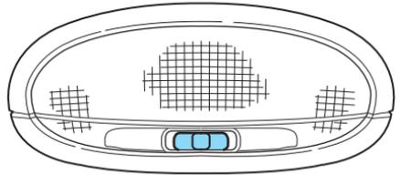
The rear dome lamp can be turned on or off by sliding the control.
