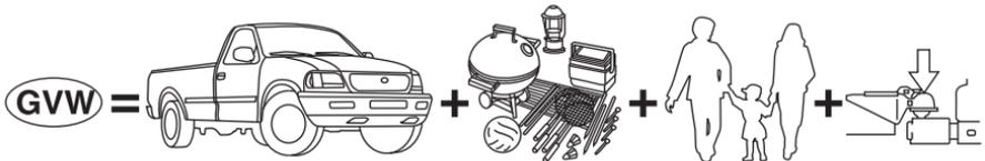
**GVW (Gross Vehicle Weight)** – is the Vehicle Curb Weight + cargo + passengers.
