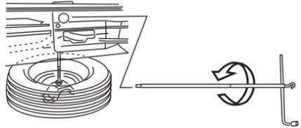
3. Turn the handle counterclockwise until tire is lowered to the ground, the tire can be slid rearward and the cable is slightly slack.
