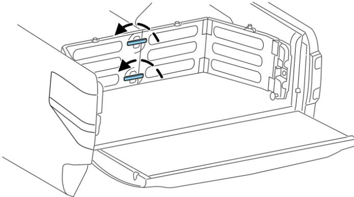
To open the bed extender into grocery mode, follow Steps 1–4 by rotating the panels away from the tailgate. Close the tailgate.
