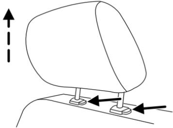
To reinstall the adjustable head restraint, do the following:
