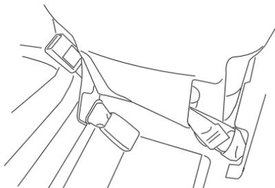
Before a passenger sits in the front center seat, make sure the lap belt and buckle are both placed in their in-use position, and no longer stowed. Always fasten your seat belt when riding in the front center seat.
