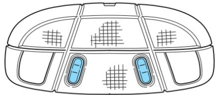
The reading portion, the two outer lights, can only be turned on and off at the lamp.
