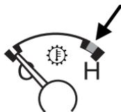
*information* for instructions. Operating the transmission for extended periods of time with the gauge in the yellow area may cause internal transmission damage.
