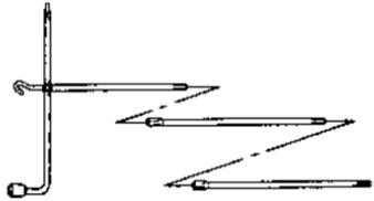
2. Fully insert the jack handle through the bumper hole and into the guide tube through the access hole in the rear bumper.
