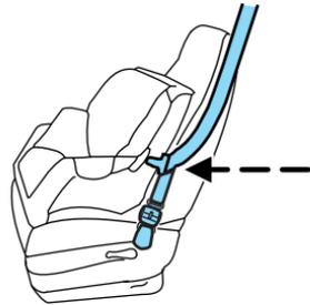
5. Insert the belt tongue into the proper buckle (the buckle closest to the direction the tongue is coming from) for that seating position until you hear a snap and feel the latch engage. Make sure the tongue is latched securely by pulling on it.
