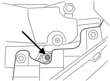
6. HORIZONTAL AIM IS NOT REQUIRED FOR THIS VEHICLE AND IS NON-ADJUSTABLE.
