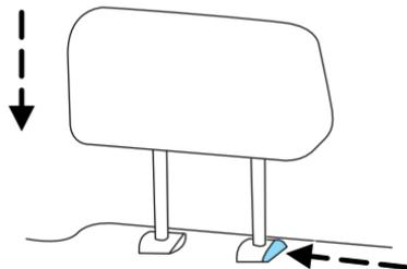
Properly adjust the head restraint so that the top of the head restraint is even with the top of your head and positioned as close as possible to the back of your head. For occupants of extremely tall stature, adjust the head restraint to its full up position.
