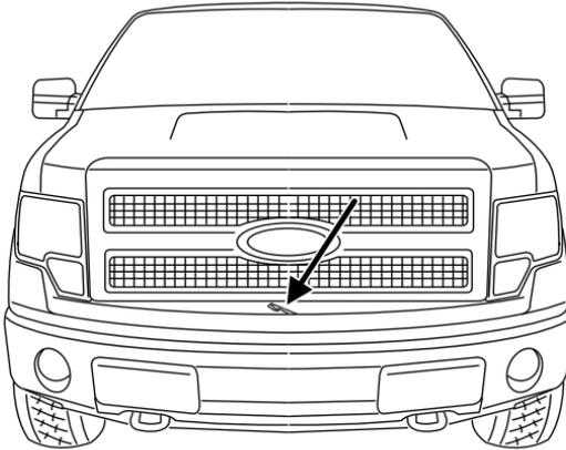
2. Go to the front of the vehicle and release the auxiliary latch that is located on the front bumper under the grill.
