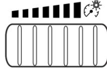
**Note:** If the battery is disconnected, discharged, or a new battery is installed, the dimmer switch requires re-calibration. Rotate the dimmer switch from the full dim position to the full dome/on position to reset. This will ensure that your displays are visible under all lighting conditions.
