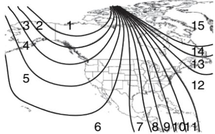
3. Press and hold the 7 and 9 radio preset buttons together for approximately five seconds until ZONE XX appears in the CID.
