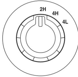
If **SHIFT DELAYED PULL FORWARD** is displayed in the message center, transfer case gear tooth blockage is present. To alleviate this condition, place the transmission in a forward gear, move the vehicle forward approximately 5 feet (1.5 m), and shift the transmission back to neutral to allow the transfer case to complete the range shift.
