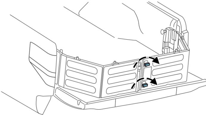
4. Connect the two panels, then rotate both knobs a quarter-turn clockwise to secure the panels.
