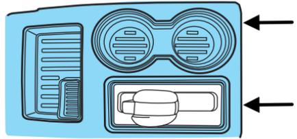
3. Locate the brake shift interlock lever on the passenger side of the shifter assembly.
