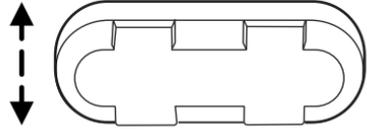
Move the switch in the direction of the arrows to raise or lower the rear portion of the seat cushion.
