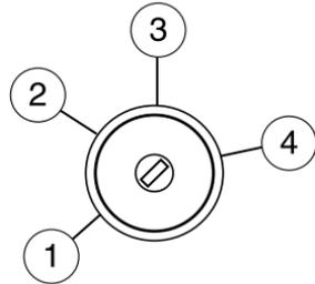
**Note:** Cranking may be stopped at any time by turning the key to the off position.
