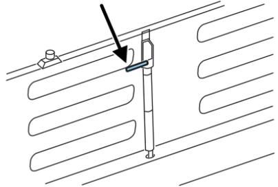
**Note:** When the vehicle is in motion, ensure the locking pins and knobs are fully engaged.
