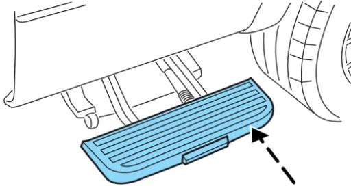
To stow the box side step, with your foot, push the box side step under the truck until fully latched. Do not push on the button while stowing the box side step.
