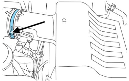
4. Pull the air tube off from the air cleaner housing.
