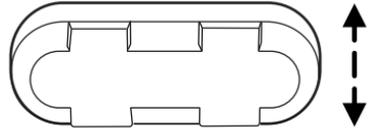
Press the switch in the direction of the arrows to move the seat forward, backward, up or down.
