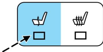
The heated seat module resets at every ignition run cycle. While the ignition is in the on position, activating the high or low heated seat switch enables heating mode. When activated, they will turn off automatically when the engine is turned off.
