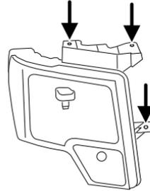
4. Once the three retaining bolts have been removed, slide the headlamp assembly forward, disconnecting the two snap attachments at the fender.
