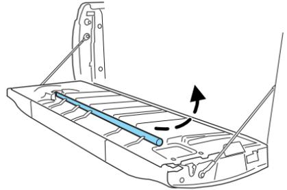
3. Rotate the center molding to unlatch the tailgate step and pull it towards you to extend it.
