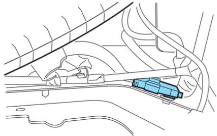
2. Install a protective cap (located in the glove box) onto the in-line rearview camera system connector that remains under the pickup box.
