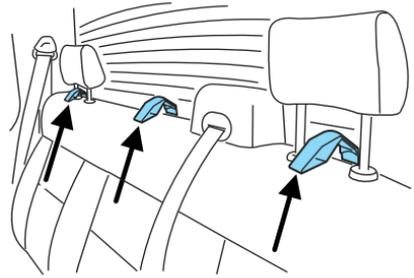
Many tether straps cannot be tightened if the tether strap is hooked to the loop directly behind the child seat. To provide a tight tether strap:
