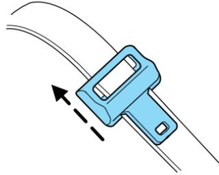
4. While holding both shoulder and lap portions next to the tongue, route the tongue and webbing through the child seat according to the child seat manufacturer's instructions. Be sure that the belt webbing is not twisted.
