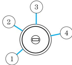
4. After three seconds but within 10 seconds of turning the ignition to the 1 (off) position, insert the second previously **coded key** into the ignition.
