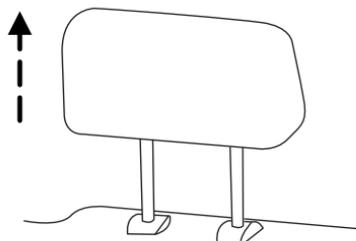
2. Lower the head restraint by pressing and holding the guide sleeve adjust/release button and pushing down on the head restraint.
