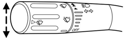
Push and hold up or down to the first detent to signal a lane change.
