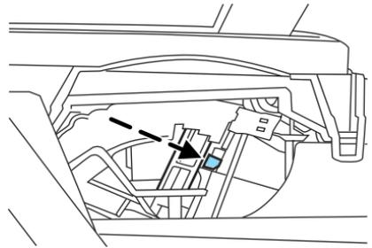
4. Apply the brake pedal. Using a screwdriver (or similar tool), press and hold the brake shift interlock lever while pulling the gearshift lever out of the P (Park) position and into the N (Neutral) position.
