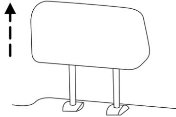
2. Simultaneously press and hold both the adjust/release button and the unlock/remove button, then pull up on the head restraint.
