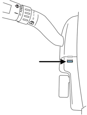
4. Insert a flat head screwdriver into each slot to unsnap and remove the steering column cover. Rotate the column up on its hinges and pull rearward to remove the cover from the hinges.
