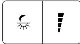
The lights come on whenever the ignition is in either the on or accessory position and the headlamps or parking lamps are on.
