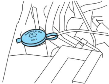
State or local regulations on volatile organic compounds may restrict the use of methanol, a common windshield washer antifreeze additive. Washer fluids containing non-methanol antifreeze agents should be used only if they provide cold weather protection without damaging the vehicle's paint finish, wiper blades or washer system.
