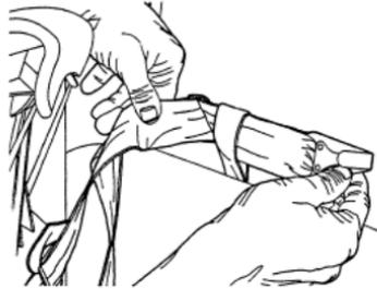
2. Route the tether strap behind the head restraint supports to a loop behind an adjacent seating position, and hook the strap hook onto the loop. If using the driver's side, pass the strap behind the shoulder belt mounting for the center seat.
