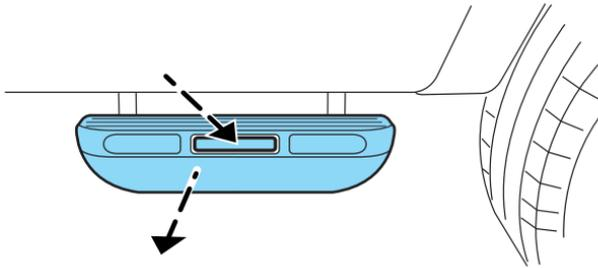
To deploy the box side step, with your foot, push down on the button. The step will automatically extend out from the stowed position.
