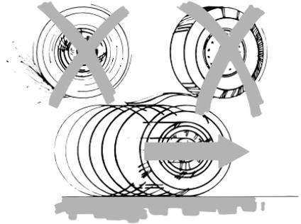
If your vehicle has anti-lock brakes, apply the brakes steadily. Do not “pump” the brakes.
