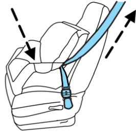
7. Allow the safety belt to retract and remove any slack in the belt to securely tighten the child safety seat in the vehicle.
