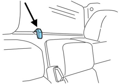
If the tether strap is clipped incorrectly, the child safety seat may not be retained properly in the event of a collision.
