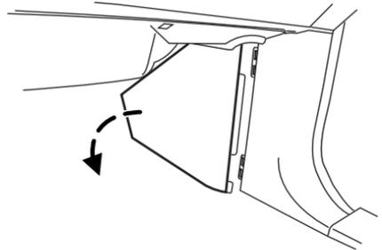
To remove the fuse box cover, press in the tabs on both sides of the cover, then pull the cover off.
