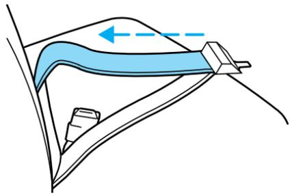
For long term storage, the lap belt can be placed into a pocket found on the inside lid of the storage compartment. To store the lap belt, do the following:
