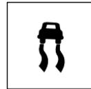
the instrument cluster will illuminate if a driving situation causes the AdvanceTrac® with RSC® system to operate. If the stability control light illuminates steadily, verify that the AdvanceTrac® with RSC® system is not manually disabled by pressing the traction control button located on the center stack of the instrument panel. If the stability control light remains steadily illuminated, have the system serviced by an authorized dealer immediately.
