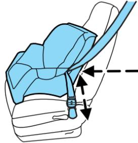
10. Check from time to time to be sure that there is no slack in the lap/shoulder belt. The shoulder belt must be snug to keep the lap belt tight during a collision.
