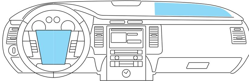
The airbag supplemental restraint system (SRS) is designed to work in conjunction with the safety belts to help protect the driver and front outboard passenger from certain upper body injuries. The term “supplemental restraint” means the airbags are intended as a supplement to the safety belts. Airbags offer the most protection when used with safety belts for crash conditions for which airbags are designed to deploy. Airbags do not offer any protection in crashes for which they do not deploy.
