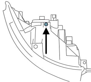
5. Locate the vertical adjuster on each headlamp. Using a Phillips #2 screwdriver, turn the adjuster either clockwise (to adjust down) or counterclockwise (to adjust up). The horizontal edge of the brighter light should touch the horizontal reference line.
