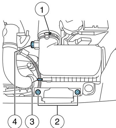
C. Remove the bolt cover (if equipped).
