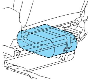
To replace the temporary mobility kit, open the Velcro® strap on the bag and slide the bag back under the driver's seat. Wrap the strap over the rear frame bar, loop it through the buckle and secure the bag to the seat frame.
