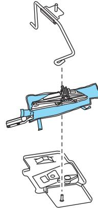
**If you are stowing the flat tire,** remove the L-shaped bolt from from the external pocket of the felt bag. With the 3rd row seat in the raised position, stand the flat tire in the rear of the vehicle with the tire's valve stem facing the rear of the vehicle. Fasten the flat tire to the vehicle by inserting the L-shaped bolt through one of the lug bolt holes in the wheel and turning clockwise into the threaded hole in the vehicle until the tire is secured.
