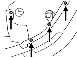
After removing to allow free access to the front fog lamp bulb and electrical wire harness, the splash shield flap should be able to be repositioned.
