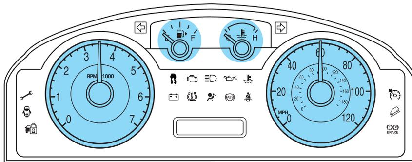
**Speedometer:** Indicates the current vehicle speed.
