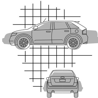
As a result of the above dimensional differences, crossover vehicles often will have a higher center of gravity and a greater difference in center of gravity between the loaded and unloaded condition.
