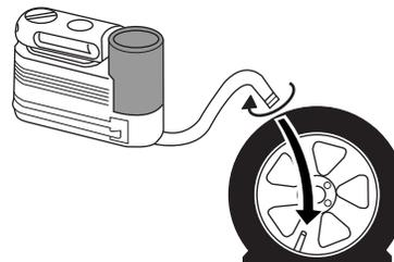
**Note: When the sealing compound is first added into the tire, the air pressure gauge reading on the compressor unit may indicate a higher value; this is normal and should be no reason for concern. The pressure will drop after about 30 seconds of operation. The**
