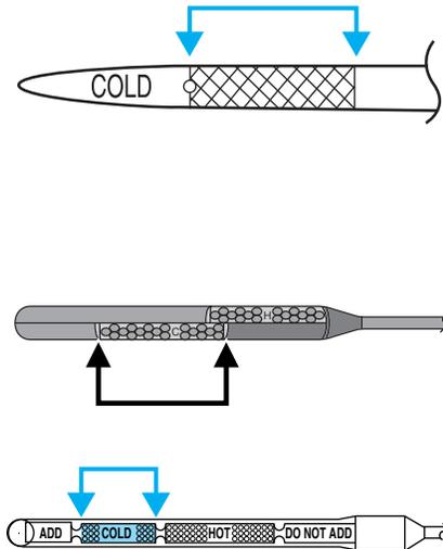
The transmission fluid should be in this range if at ambient temperature (50°F-95°F [10°C-35°C]).
