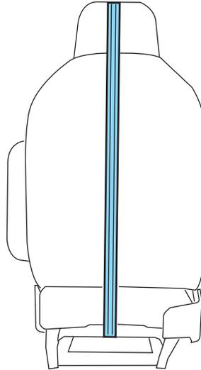
3. Clip the tether strap hook to the seat pedestal at the location shown. If the tether strap is clipped incorrectly, the child safety seat may not be retained properly in the event of a collision.
