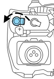
3. Rotate the bulb socket counterclockwise and remove.
