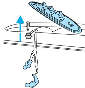
To install the new bulb, follow the removal procedure in reverse order.
