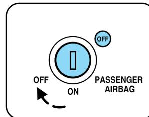
**WARNING:** If the light fails to illuminate when the passenger air bag switch is in the OFF position and the ignition switch is in ON, contact your authorized dealer as soon as possible.
