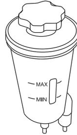
4. Check the fluid level in the reservoir. It should be between the MIN and MAX lines. Do not add fluid if the level is in this range.
