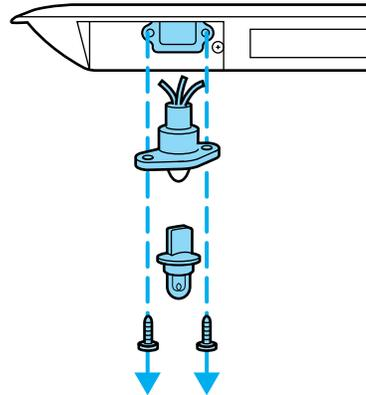
To install the new bulb, follow the removal procedures in reverse order.
