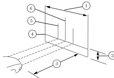
2. The center of the headlamp is marked either on the lens (a circle or cross marker) or on the bulb shield, internal to the lamp (mark or feature). Measure the height from the center of your headlamp to the ground (2) and mark an 8 foot (2.4 meter) long horizontal line on the wall or screen (1) at this height (masking tape works well).
