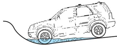
Once through water, always try the brakes. Wet brakes do not stop the vehicle as effectively as dry brakes. Drying can be improved by moving your vehicle slowly while applying light pressure on the brake pedal.
