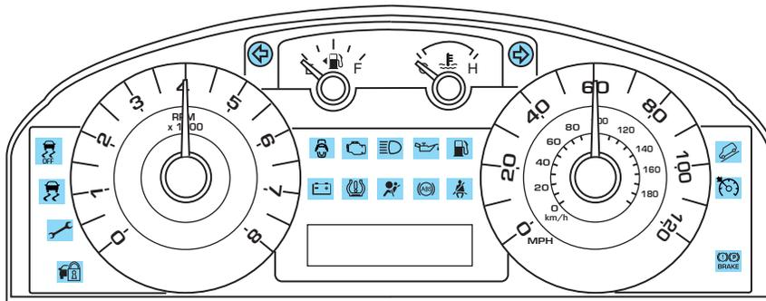
Warning lights and gauges can alert you to a vehicle condition that may become serious enough to cause extensive repairs. A warning light may illuminate when a problem exists with one of your vehicle's functions.
