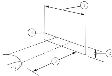
2. Measure the height from the center of your headlamp to the ground and mark an 8 foot (2.4 meter) horizontal reference line on the vertical wall or screen at this height (a piece of masking tape works well). The center of the lamp is marked by a 3 mm circle on the headlamp lens.
