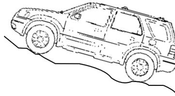
Apply just enough power to the wheels to climb the hill. Too much power will cause the tires to slip, spin or lose traction, resulting in loss of vehicle control.
