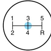
**Note:** The gearshift lever can only be moved into R (Reverse) by moving it from left of 3 (Third) and 4 (Fourth) before shifting into R (Reverse). This is a lockout feature that protects the transmission from accidentally being shifted into R (Reverse) from 5 (Fifth).
