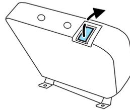
5. Rotate seatback down into load floor position.
