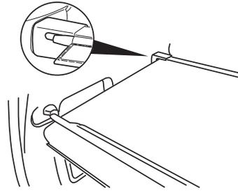
**!** **WARNING:** Ensure that the posts are properly latched in mounting features. The cover may cause injury in a sudden stop or accident if it is not securely installed.
