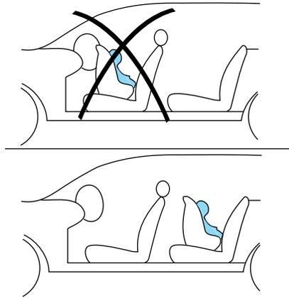
**!** **WARNING:** Airbags can kill or injure a child in a child seat. **NEVER** place a rear-facing child seat in front of an active airbag. If you must use a forward-facing child seat in the front seat, move the seat all the way back.
