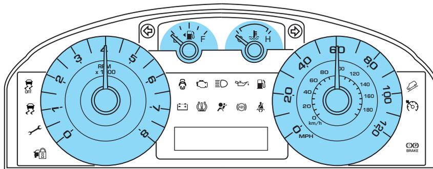
**Speedometer:** Indicates the current vehicle speed.
