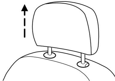
2. Simultaneously press and hold both the adjust/release button and the unlock/remove button, then pull up on the head restraint.
