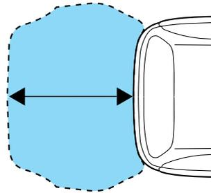
While receiving a warning the radio volume will be reduced to a predetermined level. After the warning goes away, the radio will return to the previous value. The RSS automatically turns on when the gearshift lever is placed in R (Reverse) and the ignition is on. A control in the message center allows the driver to disable the system, refer to *Message center* in the *Instrument Cluster* chapter for more information.
