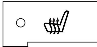
The heated seats will activate when the ignition is in the on position and the engine is running.
