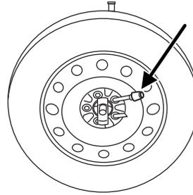
6. If not replacing the spare or flat tire to the underbody storage area, raise winch up into the installed position.
