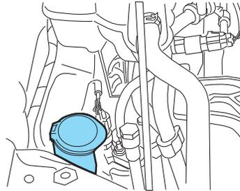
Only use a washer fluid that meets Ford specifications. Do not use any special washer fluid such as windshield water repellent type fluid or bug wash. They may cause squeaking, chatter noise, streaking and smearing. Refer to the *Maintenance product specifications and capacities* section in this chapter.
