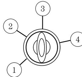
2. Turn the key to 4 (start), then release the key as soon as the engine begins cranking. Your vehicle has a computer assisted cranking system that assists in starting the engine. After releasing the key from the 4 (start) position, the engine may continue cranking for up to 10 seconds or until the vehicle starts.
