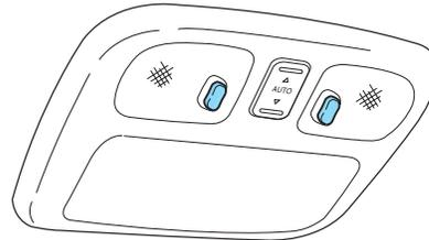
**Note:** The dome lamp and map lamps are preset to illuminate when a door is opened and will remain on for 25 seconds after the door is closed.
