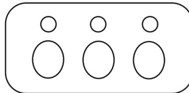
1 second) release the button once the garage door moves. When the button is released, the indicator light will begin to blink rapidly until programming is complete.
