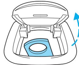
4. Clip the tether strap to the anchor as shown.
