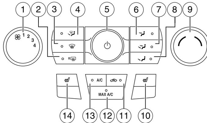
1. **Fan speed adjustment:** Controls the volume of air circulated in the vehicle.
