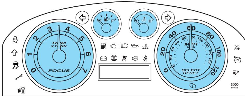
**Speedometer:** Indicates the current vehicle speed.
