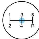
4. Press the brake pedal and move the gearshift lever to the desired gear; 1 (First) or R (Reverse).
