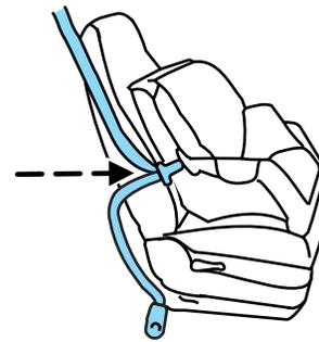
4. Insert the belt tongue into the proper buckle for that seating positions until you hear a snap and feel it latch. Make sure the tongue is securely latched to the buckle by pulling on the tongue.
