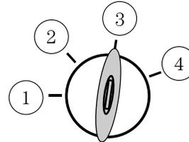
2. Accessory—allows the electrical accessories such as the radio to operate while the engine is not running.
