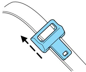
3. Provide enough lap belt length so that the tongue can reach the buckle.
