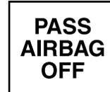
**Note:** The indicator lamp will illuminate for a short period of time when the ignition is turned to the on position to confirm it is functional.
