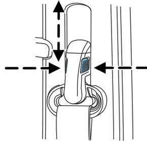
**!** **WARNING:** Position the safety belt height adjusters so that the belt rests across the middle of your shoulder. Failure to adjust the safety belt properly could reduce the effectiveness of the seat belt and increase the risk of injury in a collision.
