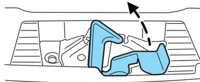
3. Lift the hood and locate the prop rod on the passenger side of the vehicle near the fender. Support the hood with the prop rod.
