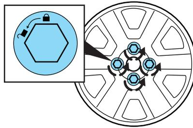
3. Loosen each wheel lug nut one-half turn counterclockwise but do not remove them until the wheel is raised off the ground.
