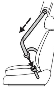
3. Allow the belt to retract. As the belt retracts, you will hear a clicking sound. This indicates the safety belt is now in the automatic locking mode.
