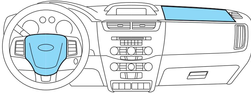
The supplemental restraint system is designed to work with the safety belt to help protect the driver and right front passenger from certain upper body injuries.
