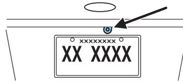
To use the camera system, place the transmission in R (Reverse); an image will display in the rearview mirror or on the navigation screen (if equipped). The area displayed on the screen may vary according to the vehicle orientation and/or road condition.
