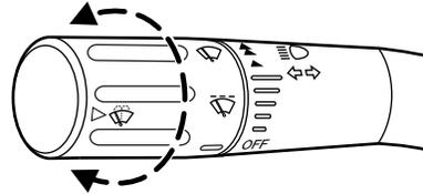
**Speed dependent wipers (if equipped):** When the wiper control is set to any of the interval settings except the longest pause setting, the pause time between wiping will automatically adjust with the vehicle speed. The faster your vehicle is travelling the shorter the pause time between wipes will become.
