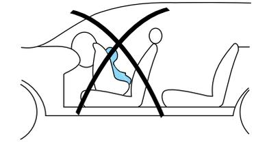
**!** **WARNING:** Airbags can kill or injure a child in a child seat. **NEVER** place a rear-facing child seat in front of an active airbag. If you must use a forward-facing child seat in the front seat, move the seat all the way back.
