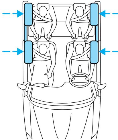
Side air curtains and side airbags, in combination with safety belts, can help reduce the risk of severe injuries in the event of a significant side impact collision.
