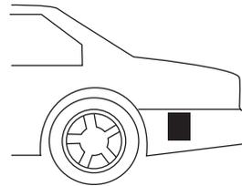
driver via the message center. If condition is determined by the system, the message center displays BLIND SPOT NOT AVAILABLE or CROSS TRAFFIC NOT AVAILABLE warning and the appropriate left and/or right exterior mirror alert indicator will illuminate. The message center warning may be cleared by the driver but the exterior mirror alert indicator will remain illuminated.
