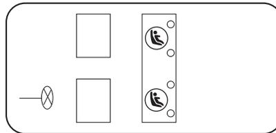
The LATCH anchors are located at the rear section of the rear seat between the cushion and seat back, below the locator symbols on the seat back. Follow the child seat manufacturer's instructions to properly install a child seat with LATCH attachments.
