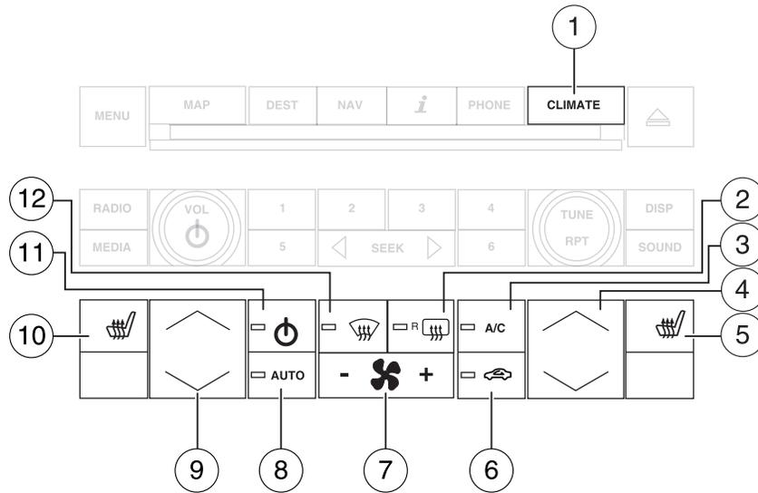
1. **CLIMATE:** Press to control the climate control system through the touch display screen. See *Touchscreen functions* later in this section.
