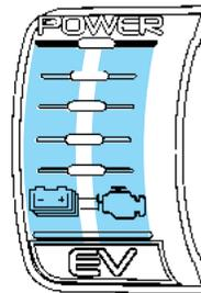
Maximum displayed gasoline engine power is greater than the maximum displayed battery power.
