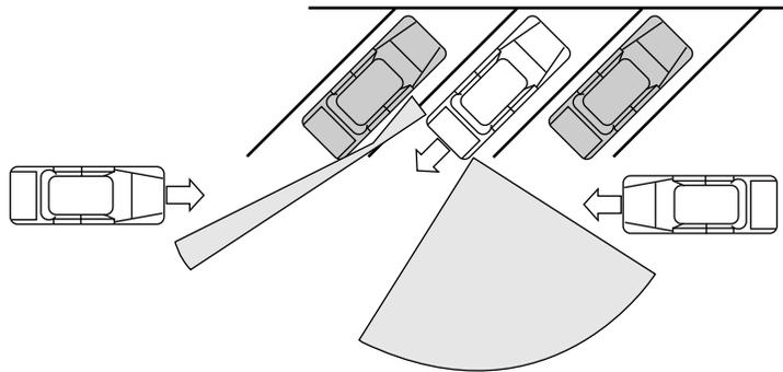
**CTA detection limitations:** Due to the nature of radar technology, there may be certain instances where vehicles entering and exiting the blind spot zones may not be detected. Below is a list of circumstances that may cause non detection:
