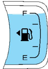
The fuel icon with the arrow points to the side of the vehicle that the fuel filler door is on.
