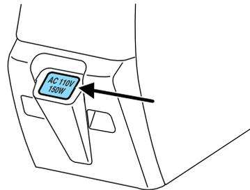
**Note:** The 110V AC power point is equipped with a safety cap and a safety twist tab. They both provide protection from inserting any object into the power point other than the 110V AC electrical device plug. The safety cap should always be in a closed position whenever the power point outlet is not in use.
