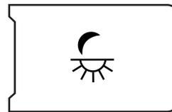
The lights come on whenever the ignition is in either the on or accessory position.
