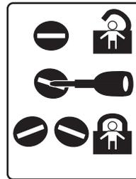
The childproof locks are located on the rear edge of each rear door and must be set separately for each door. Setting the lock for one door will not automatically set the lock for both doors.
