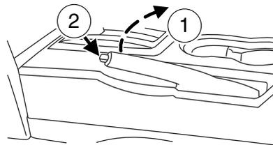
The BRAKE warning lamp will illuminate and will remain illuminated until the parking brake is released.
