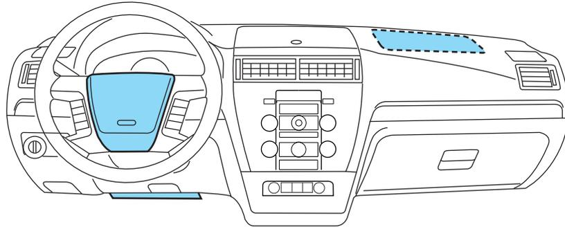
The passenger airbag cover is a seamless design so that you cannot see the boundary around its door. The shaded area in the illustration represents the passenger airbag cover.
