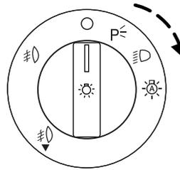
The autolamp system also keeps the lights on for a predetermined amount of time after the ignition switch is turned to off. You can change the amount of time the lamps stay on by using the programming procedure that follows:
