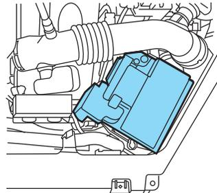
**If your battery has a cover/shield, make sure it is reinstalled after the battery has been cleaned or replaced.**
