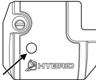
5. Locate and carefully remove the engine oil level dipstick.
