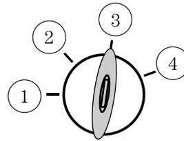
After releasing the key from the 4 (start) position, a vehicle symbol (called the Ready Indicator Light) will illuminate in the instrument cluster to indicate the vehicle is
