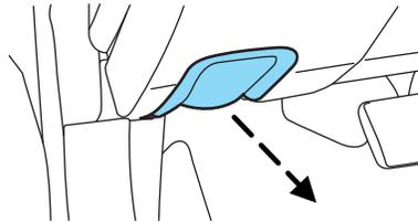
2. Go to the front of the vehicle and release the auxiliary latch that is located under the front center of the hood.
