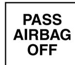
**Note:** The indicator lamp will illuminate for a short period of time when the ignition is turned to the on position to confirm it is functional.
