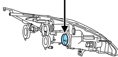
2. Turn the bulb holder counterclockwise and remove it.
