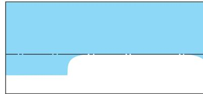
4. Locate the vertical adjuster on each headlamp. Using a Phillips #2 screwdriver or 13 mm wrench/socket, turn the adjuster either clockwise (to adjust down) or counterclockwise (to adjust up). The horizontal edge of the brighter light should touch the horizontal reference line.
