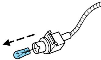
3. Reverse the procedure to install the new bulb.
