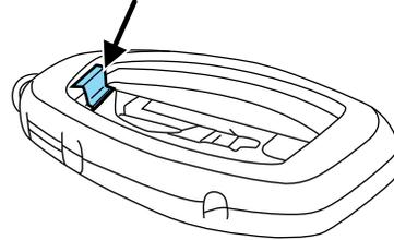
4. Carefully insert a flat object in the position shown to open the transmitter.
