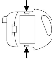
3. Carefully pry out the battery with a flat object. Be careful not to touch the battery contacts or the printed circuit board with the flat object.
