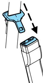
2. To unfasten, press the release button and remove the tongue from the buckle.
