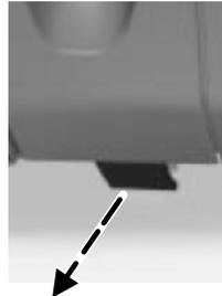
2. Raise the hood slightly. Then push the hood latch release lever, located under the front center of the hood, to the left.
