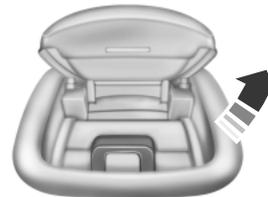
4. Clip the tether strap to the anchor as shown.
