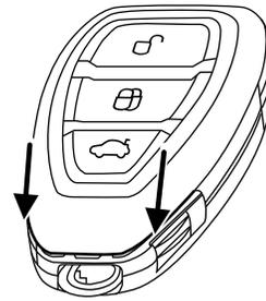
5. Carefully pry out the battery with a flat object.
