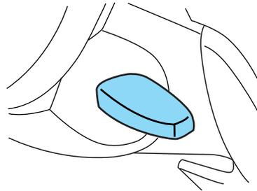
to the backup location near the steering column. After holding the IA key to the backup location, use the START/STOP button and brake pedal (automatic transmission) or clutch pedal (manual transmission) to start your vehicle as usual. The vehicle should respond normally as long as the IA key is at the backup location on the steering column. Once the vehicle is started, the IA key can be moved from the backup location, if desired.
