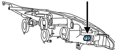
2. Remove the bulb from the bulb holder.
