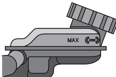
Fluid levels between the MIN and MAX lines are within the normal operating range; there is no need to add fluid.
