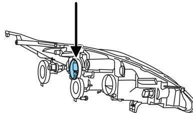
2. Turn the bulb holder counterclockwise and remove it.
