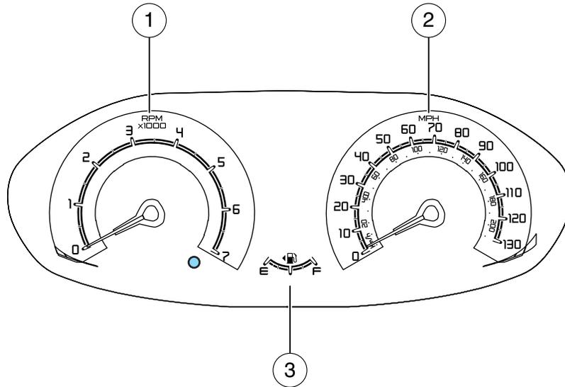
1. **Tachometer:** Indicates the engine speed in revolutions per minute. Driving with your tachometer pointer continuously at the top of the scale may damage the engine.
