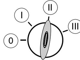
**Note:** Cranking may be stopped at any time by turning the key to the off position.
