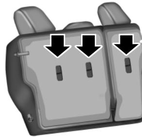
3. Clip the tether strap to the anchor as shown.
