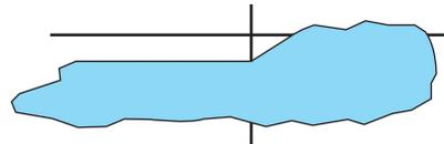
5. Locate the vertical adjuster on each headlamp. Using a Phillips #2 screwdriver, turn the adjuster either clockwise (to adjust down) or counterclockwise (to adjust up). The horizontal edge of the brighter light should touch the horizontal reference line.
