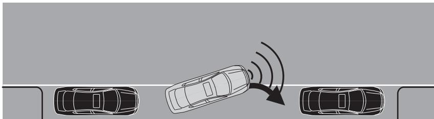
When you determine the vehicle is far enough forward or a solid tone from the forward sensing system (if equipped) is heard, bring the vehicle to a complete stop and move the gearshift to R (Reverse). The message center may display BACK UP SLOWLY USE CAUTION followed by a chime. The system may offer subsequent backward and forward maneuvers before proceeding to the finish phase.
