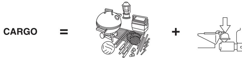
**Cargo Weight** – includes all weight added to the Base Curb Weight, including cargo and optional equipment. When towing, trailer tongue load weight is also part of cargo weight.
