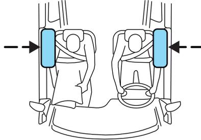
Side airbags, in combination with safety belts, can help reduce the risk of severe injuries in the event of a significant side impact collision.
