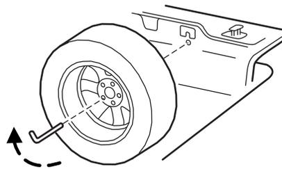
**If you are stowing the temporary spare tire,** place the tire over the jack and secure it with the large wing nut.
