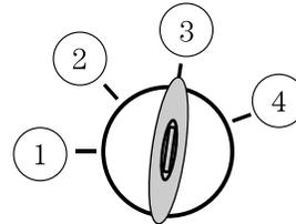
2. Turn the key to 4 (start), then release the key as soon as the engine begins cranking. Your vehicle has a computer assisted cranking system that assists in starting the engine. After releasing the key from the 4 (start) position, the engine may continue cranking for up to 10 seconds or until the vehicle starts.
