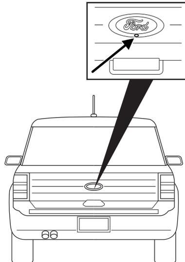
To use the camera system, place the transmission in R (Reverse); an image will display on the navigation screen. The area displayed on the screen may vary according to the vehicle orientation and/or road condition.
