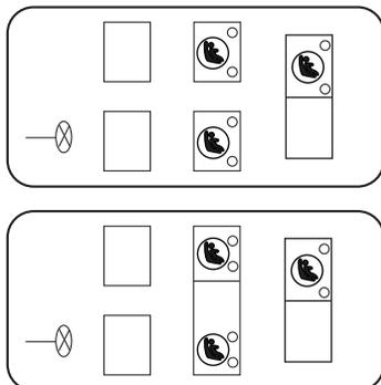
The LATCH anchors are located at the rear section of the rear seat between the cushion and seat back, below the locator symbols on the seatback. Follow the child seat manufacturer's instructions to properly install a child seat with LATCH attachments.
