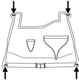
Some vehicles may be equipped with an aero-shield under the engine. This shield needs to be removed for service, including oil and filter changes. It is secured with four quick release fasteners.
