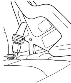
Airbags can kill or injure a child in a child seat. NEVER place a rear-facing child seat in front of an active airbag. If you must use a forward-facing child seat in the front seat, move the vehicle seat all the way back.
