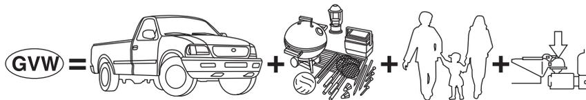
**GVW (Gross Vehicle Weight)** – is the Vehicle Curb Weight + cargo + passengers.
