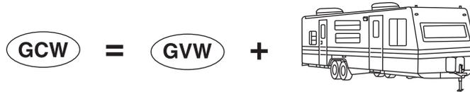
**GCW (Gross Combined Weight)** – is the weight of the loaded vehicle (GVW) plus the weight of the fully loaded trailer.
