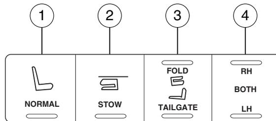
Press the seat selection button (4) to select either right-hand seat, the left-hand seat or both. First select the seat you would like to adjust, then select one of the following:
