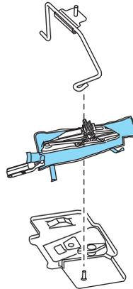
**If you are stowing the flat tire,** remove the L-shaped bolt from the external pocket of the felt bag. With the 3rd row seat in the raised position, stand the flat tire in the rear of the vehicle with the tire's valve stem facing the rear of the vehicle. Fasten the flat tire to the vehicle by inserting the L-shaped bolt through one of the lug bolt holes in the wheel and turning clockwise into the threaded hole in the vehicle until the tire is secured.
