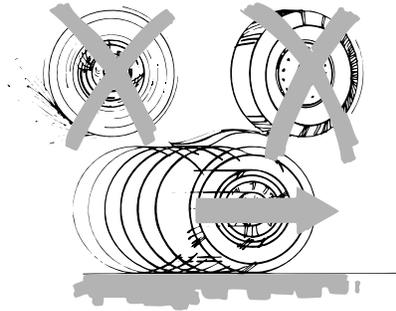
Your vehicle has anti-lock brakes, therefore apply the brakes steadily. Do not “pump” the brakes.
