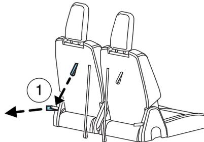
3. Release the cushion latches by pulling the number 2 strap while pulling on the strap located at the top of the seatback to tumble the seat all the way into the floor tub.
