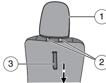
To fold the head restraint, pull the fold strap. To place the head restraint back to the upright position, pull up on the head restraint.
