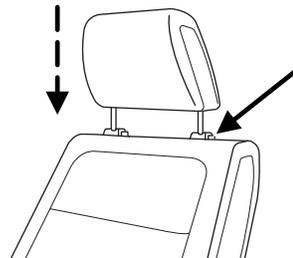
Properly adjust the head restraint so that the top of the head restraint is even with the top of your head and positioned as close as possible to the back of your head. For occupants of extremely tall stature, adjust the head restraint to its full up position.
