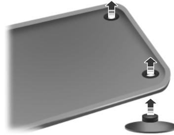
**!** **WARNING:** Always use floor mats that are designed to fit the foot well of your vehicle. Only use floor mats that leave the pedal area unobstructed. Only use floor mats that are firmly secured to retention posts so that they cannot slip out of position and interfere with the pedals or impair safe operation of your vehicle in other ways.
