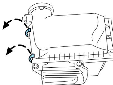
1. Release the clamps that secure the air filter housing cover.
