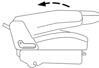
**Note:** The seatback will not raise if the rear latch hooks are not properly engaged to the floor
