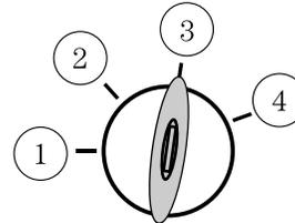
In order to switch off the engine while the vehicle is in motion, shift to neutral and use the brakes to bring the vehicle to a safe stop. After the vehicle has stopped, turn the engine off and shift into park. Then, turn the key to the accessory or off position.
