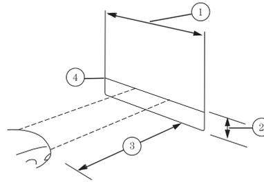
2. Measure the height of the headlamp bulb center from the ground and mark an 8 foot (2.4 meter) horizontal reference line on the vertical wall or screen at this height (a piece of masking tape works well).
