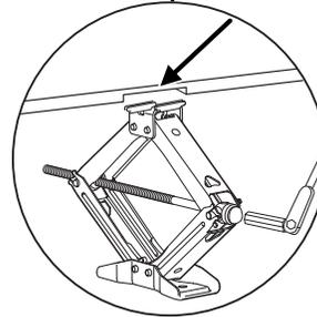
6. Lower the wheel by turning the jack handle counterclockwise.
