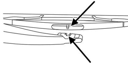
4. Attach the new wiper to the wiper arm and press it into place until a click is heard.
