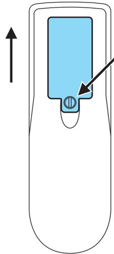
Remove the screw and unlatch the battery cover to access the batteries. The remote control unit uses two AAA batteries which are supplied with the unit.
