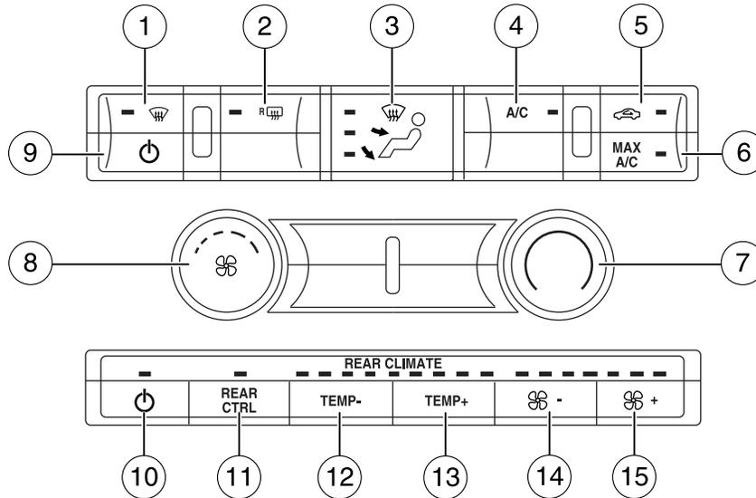
1. **Defrost:** Distributes outside air through the windshield defroster vents and demister vents. Can be used to clear the windshield of fog and thin ice. The system will automatically provide outside air to reduce window fogging. Press this button again to return to the previous air flow selection.
