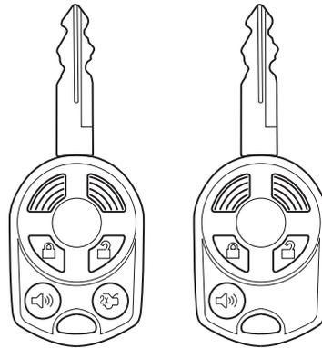
The typical operating range for your IKT is approximately 33 feet (10 meters). A decrease in operating range could be caused by:
