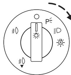
The fog lamp indicator light will illuminate when the fog lamps have been turned on. The fog lamps will not operate when the high beams are active.
