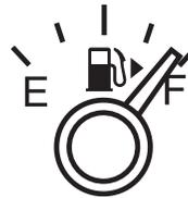
The fuel icon and arrow indicates which side of the vehicle the fuel filler door is located.
