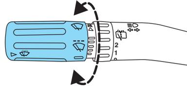
**Speed dependent wipers:** When the wiper control is set on the intermittent settings, the speed of the wipers will automatically adjust with the vehicle speed. The faster your vehicle is travelling the faster the wipers will go.
