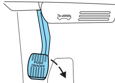
The BRAKE warning lamp in the instrument cluster illuminates and remains illuminated (when the ignition is turned on) until the parking brake is released.
