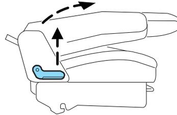
2. Lift the handle all the way up until the seat releases from the floor. Rotate the seat forward to allow access to the third row.
