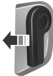
2. Go to the front of the vehicle and locate the auxiliary latch located under the front of the hood (left of center) and then release it by pushing the auxiliary latch to the right.
