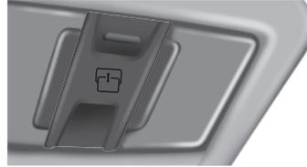
**To close the moon roof:** Press and release the front of the control.
