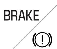
If the brake system warning light does not illuminate at this time, seek service immediately from your authorized dealer. Illumination after releasing the parking brake indicates low brake fluid level and the brake system should be inspected immediately by your authorized dealer.
