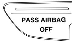
**Note:** The indicator lamp will illuminate for a short period of time when the ignition is turned to the on position to confirm it is functional.
