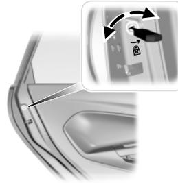
The childproof locks are located on the rear edge of each rear door and must be set separately for each door. Setting the lock for one door will not automatically set the lock for both doors.
