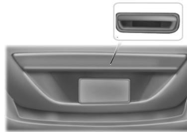
1. Unlock the trunk with the remote control or power door lock control. The trunk will unlock when you press the release button if the intelligent access transmitter is within 3 feet (1 meter) of the trunk.
