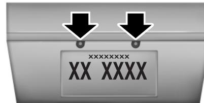
The rear video camera system, located on the liftgate above the license plate, provides a video image of the area behind the vehicle.
