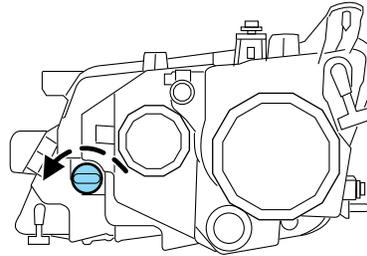
5. Carefully pull bulb straight out of socket and push in the new one.
