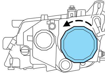
4. Remove the bulb socket by rotating it counterclockwise, then pull it straight out of the lamp assembly.
