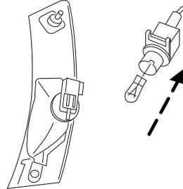
Replace with a new bulb, and reverse the removal steps to complete the process.
