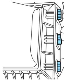
3. Remove the air filter element from the air filter housing.
