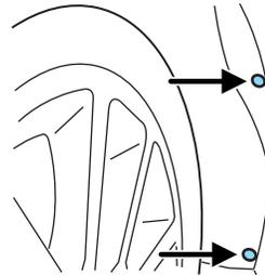
3. Reaching through the wheel well, remove the rubber headlamp bulb access cover.
