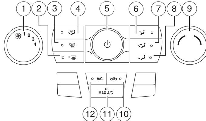
1. **Fan speed adjustment:** Turn to select fan speed.
