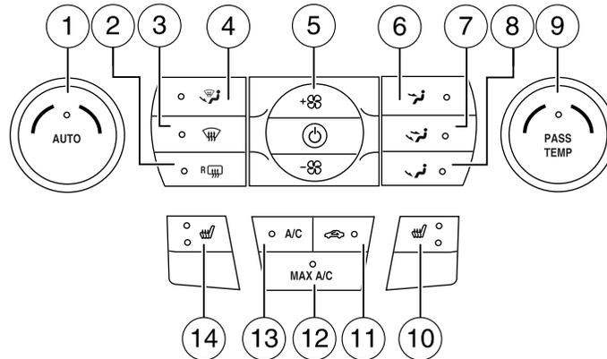
1. **AUTO/Driver temperature:** Press to engage full automatic operation. Select the desired temperature using the temperature control.
