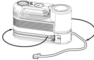
2. Press the button located on the temporary mobility kit compressor housing below the canister while pulling up on the sealant canister.
