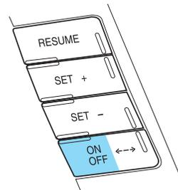
3. Press and release the SET + control. The vehicle speed will be stored in the memory and the message center will display SET XXX MPH (your desired speed).
