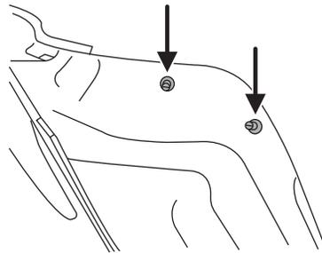
3. Remove the nut and washer assemblies, then pull the lamp assembly away from the vehicle.
