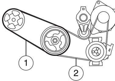
1. Short drivebelt is on first pulley groove closest to engine (except vehicles with electric power assisted steering).
