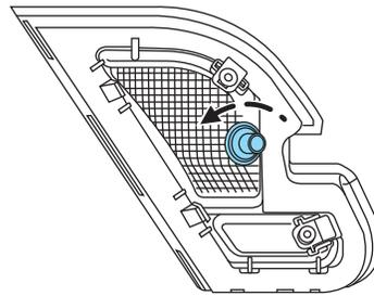
4. Disconnect the wire harness connector from the bulb/socket.
