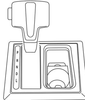
4. Insert the screwdriver (or similar tool) into the access hole and press while pulling the gearshift lever out of the P (Park) position and into the N (Neutral) position.
