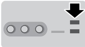
The ports are located either in the center console or behind a small access door in the instrument panel. To access and play music from your device, press the lower left corner of the touchscreen, and then select the **USB** tab.
