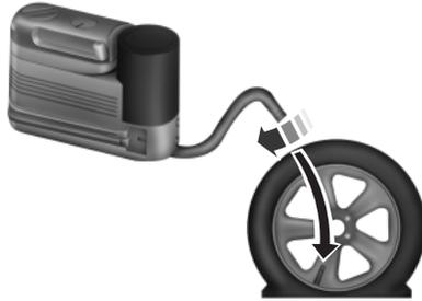
8. Inflate the tire to the pressure listed on the Tire Label located on the driver's door or the door jamb area.
