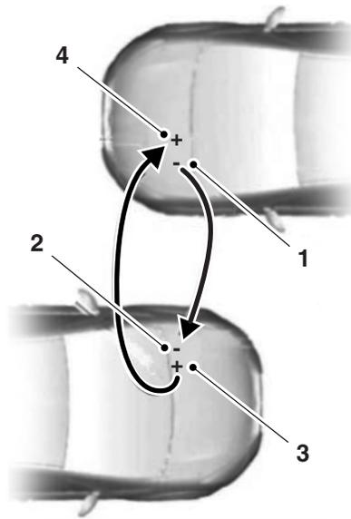
1. Remove the jumper cable from the negative (-) prong on your vehicle's battery.
