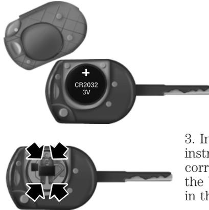
1. Twist a thin coin in the slot of the transmitter near the key ring to remove the battery cover.
