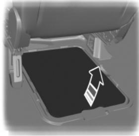
The under floor storage compartments are located in front of the rear seats. Make sure the lids are secure before driving.
