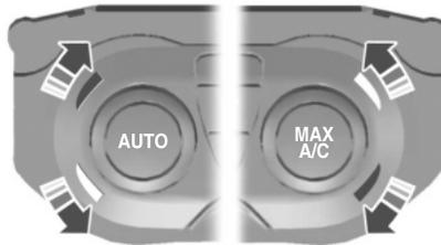
You can set the temperature between 60°F (15.5°C) and 85°F (29.5°C) in 1°F (0.5°C) increments. In position LO, 59°F (15°C), the system switches to permanent cooling. In position HI, 86°F (30°C), the system switches to permanent heating.
