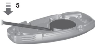
**Note:** Do not touch the battery contacts or the printed circuit board with the screwdriver.
