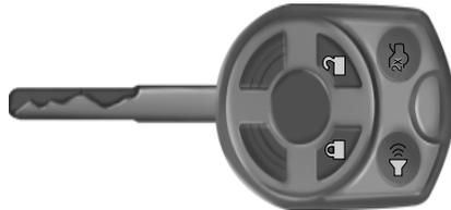
Your vehicle may be equipped with two integrated keyhead transmitters. Use the key blade to start your vehicle and unlock or lock the driver door from outside the vehicle. The transmitter portion functions as the remote control.
