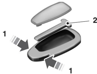
1. Press and hold the push buttons to release the cover. Carefully remove the cover.
