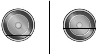
If driving through deep or standing water is unavoidable, proceed very slowly. Never drive through water that is higher than the bottom of the wheel rims (for cars) or the bottom of the hubs (for trucks).
