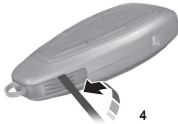
4. Twist the screwdriver in the position shown to separate the two halves of the remote control.
