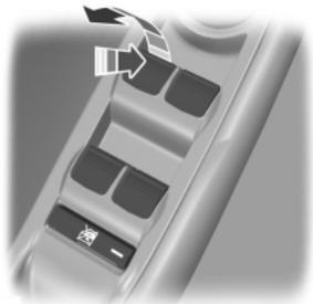
Press the switch to open the window.
