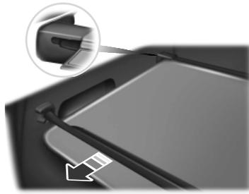
Insert the ends of the cargo shade into the mounting features located behind the rear seat on the rear trim panels to install the shade.
