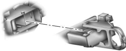
4. Pull the handle toward you and remove the circuit from the vehicle to disable the high-voltage battery.
