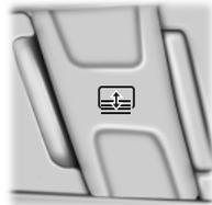
Fully press and release the front of the control to open the sun shade.
