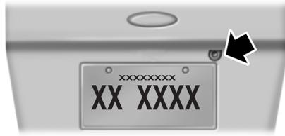
The camera is located on the liftgate.
