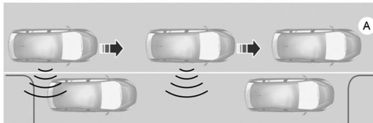
When a suitable space is found, the touch screen displays a message and a chime sounds. Slow down and stop at approximately position (A), then follow the instructions on the touch screen.
