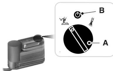
7. Push and turn dial (A) counterclockwise to the sealant position. Turn on the kit by pressing the on button (B).
