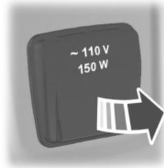
The power point is used for powering electrical devices that require up to 150 watts. It is located on the rear of the center console.
