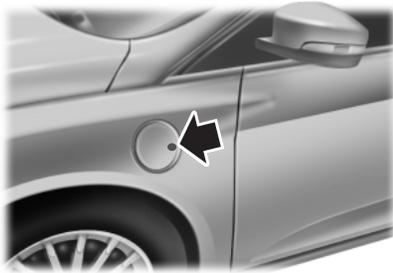
The charge port is located between the front left side door and front left wheel well. There is an indentation located on the charge port door. Press with your thumb to press to open and close the door.
