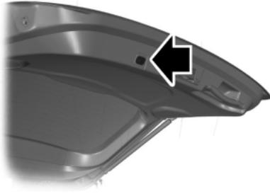
**To close with the control on the liftgate:** Press and release the button.
