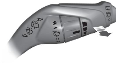
The washer will spray for as long as the lever is pulled toward you. After you release the lever, the wipers will operate for a short time.
