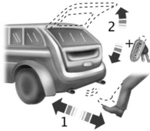
1. Make sure you have an intelligent access transmitter within 3 feet (1 meter) of the liftgate.
