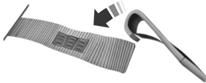
4. Tighten the child safety seat tether strap according to the manufacturer's instructions.
