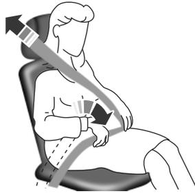
Pregnant women should always wear their safety belts. The lap belt portion of a combination lap and shoulder belt should be positioned low across the hips below the belly and worn as tight as comfort will allow. The shoulder belt should be positioned to cross the middle of the shoulder and the center of the chest.
