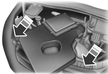
5. Lift the air cleaner assembly (A) from the mounting studs, then rotate and pull it towards the front of the vehicle.
