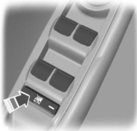
Press the control to lock or unlock the rear window controls. It illuminates when you lock the rear window controls.
