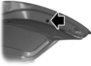
The new open liftgate height will now be recalled when the power liftgate is opened. To change the programmed height, repeat the above procedure. Once the power liftgate is opened it can be manually moved to a different height.
