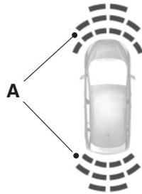
A. Coverage area of up to 27 inches (70 centimeters) from the front of the vehicle and about 6–14 inches (15–35 centimeters) to the side of the front end of the vehicle. Refer to the reverse sensing section for details on coverage area.
