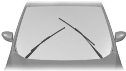
4. Release the lever when the wipers have moved to the service position.
