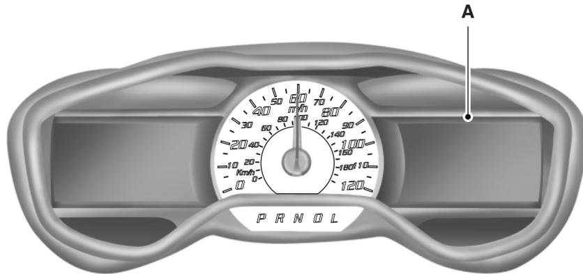
The display is located on the right side of your instrument cluster. You can use your steering wheel controls to view and make minor adjustments to active modes without taking your hands off the wheel. For example:
