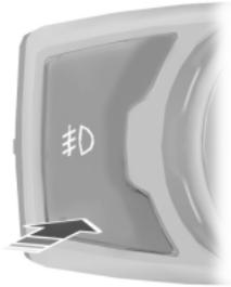
Press the control to switch the fog lamps on or off.
