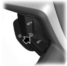
The cruise controls are located on the steering wheel.
