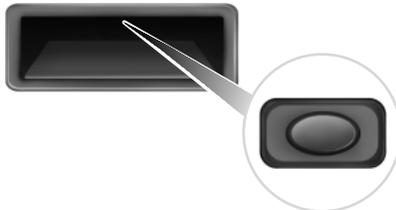
**To open the liftgate:** Press the button located in the top of the liftgate pull cup handle to unlatch the liftgate, then pull on the outside handle.
