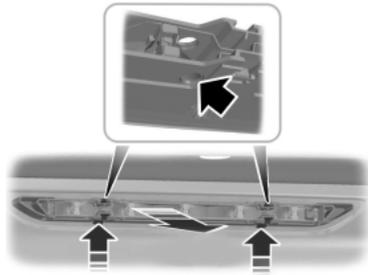
3. Insert a suitable tool into the holes.
