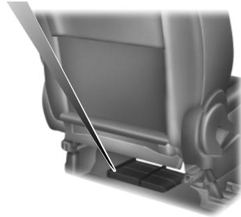
The temporary mobility kit consists of an air compressor to reinflate the tire and a sealing compound in a canister that will seal most punctures caused by nails or similar objects. This kit will provide a temporary seal allowing you to drive your vehicle up to 120 miles (200 kilometers) at a maximum speed of 50 mph (80 km/h).
