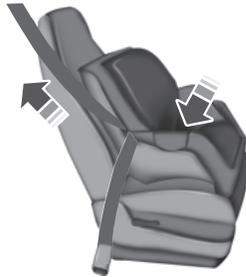
8. Remove remaining slack from the belt. Force the seat down with extra weight, for example, by pressing down or kneeling on the child restraint while pulling up on the shoulder belt in order to force slack from the belt.
