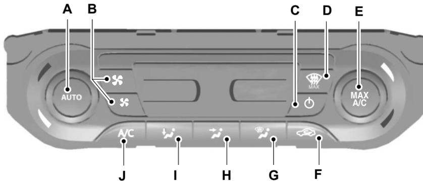
A. **AUTO:** Press to select automatic operation. The system automatically controls the temperature, amount and distribution of the airflow to reach and maintain your previously selected temperature.
