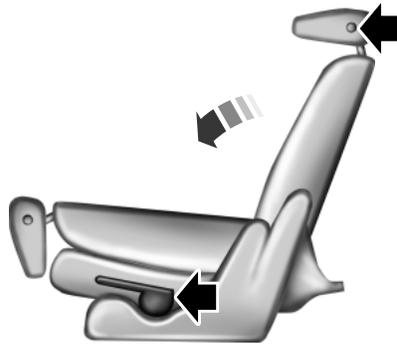
1. Press the button on the outboard side of each rear outboard headrest to fold them. Make sure the rear center headrest is in the full down position.
