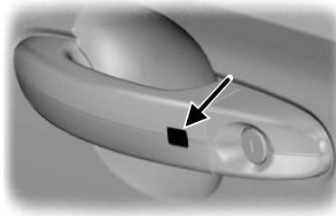
Press and hold the door handle lock sensor to lock your vehicle. To avoid unlocking the door inadvertently, be sure to only touch the lock sensor and not other areas of the door handle.
