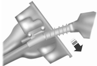
4. Slowly insert the fuel filler nozzle fully into the fuel system, and leave the nozzle fully inserted to open both doors until you are done pumping. Hold handle higher during insertion for easier access.
