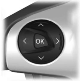
Press the OK button to acknowledge and remove some messages from the information display. Other messages will be removed automatically after a short time. Certain messages need to be confirmed before you can access the menus.
