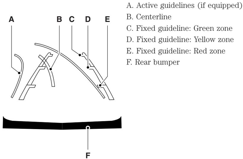
If your vehicle is equipped with active guidelines they are only shown with fixed guidelines. To use active guidelines, turn the steering wheel to point the guidelines toward an intended path. If the steering wheel position is changed while reversing, the vehicle might deviate from the original intended path.
