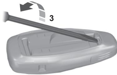
3. Twist the screwdriver in the position shown to start separating the two halves of the remote control.
