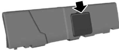
2. Remove the cover panel. A cut out area will be visible which allows your hand access to the circuit.
