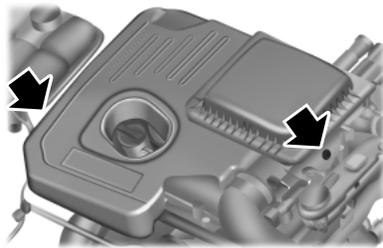
4. Remove the bolts from each side of the air cleaner assembly (A) as shown with arrows.
