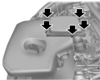
6. Loosen the 5 bolts from the air cleaner cover (B).
