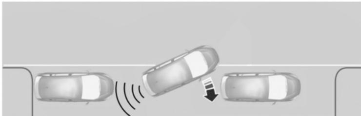
When automatic steering is finished, the touch screen displays a message indicating that the active park assist process is done. The driver is responsible for checking the parking job and making any necessary corrections before putting the transmission in P (Park).
