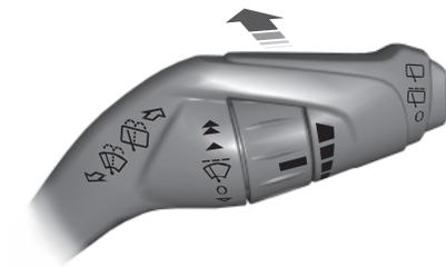
The washer will spray for as long as you push the lever away from you. When you release the lever, the wiper will operate for a short time.
