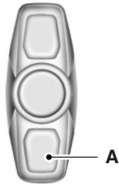
Press switch A to switch individual map lamps on and off (if equipped).
