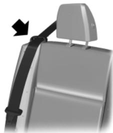
When in use, place the rear safety belts in the belt guides on the outboard seat backs.
