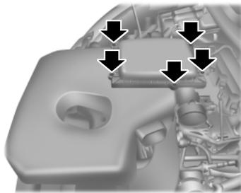
2. Install the air cleaner cover (B) and tighten the 5 bolts.
