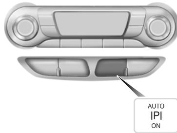
Press the button; the touch screen displays a message and a corresponding graphic to indicate it's searching for a parking space. Use the turn signal to indicate which side of the vehicle you want the system to search on.
