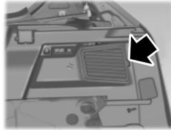
Remove the panel to access the lever.
