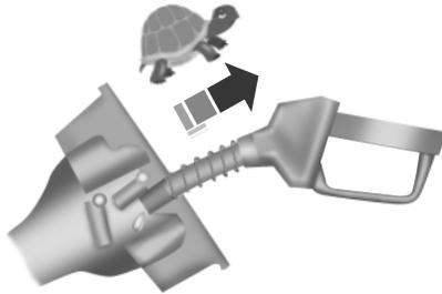
5. After you are done pumping fuel, slowly remove the fuel filler nozzle—allow about five to ten seconds after pumping fuel before removing the fuel filler nozzle. This allows residual fuel to drain back into the fuel tank and not spill onto the vehicle.
