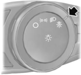
The headlamps will switch on and off automatically in low light situations or during inclement weather.
