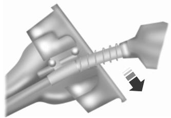
3. Slowly insert the fuel filler nozzle fully into the fuel system, and leave the nozzle fully inserted to open both doors until you are done pumping. Hold handle higher during insertion for easier access.
