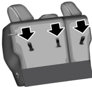
2. Locate the correct anchor on the back panel of the rear seat for the selected seating position. The anchors are labeled with the tether strap symbol.
