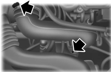
1. Loosen the hose clamps for air cleaner outlet tube (C). Disconnect the tube from the air cleaner assembly (A).
