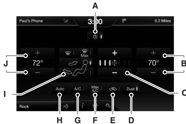
A. **Power:** Touch to switch the system off and on. Outside air cannot enter your vehicle when you switch off the system.
