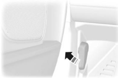
1. Inside the vehicle, pull the hood release handle located under the instrument panel.
