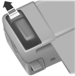
Remove the cargo shade by pressing the release lever on each side forward, then lifting the shade out of the mounting feature. You will see a red mark when the lever is unlatched.
