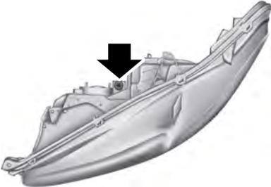
5. Locate the vertical adjuster on each headlamp. Using a Phillips #2 screwdriver, turn the adjuster either clockwise or counterclockwise in order to adjust the vertical aim of the headlamp. The horizontal edge of the brighter light should touch the horizontal reference line.
