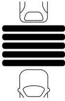
5. A lead vehicle graphic will illuminate if there is a vehicle detected in front of you.
