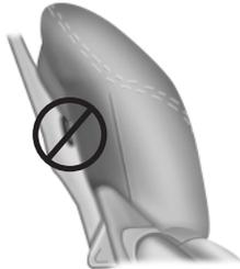
**Note:** The attachments for the convertible boot located on the back of the head restraints are not tether anchors.
