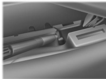
4. Press and hold the lever forward while pulling the gearshift lever out of the **P** (Park) position and into the **N** (Neutral) position.
