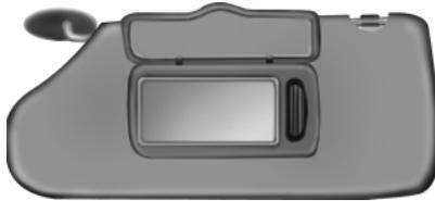
Lift the cover to switch on the lamp.
