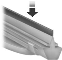
Run the tip of your fingers over the edge of the blade to check for roughness.
