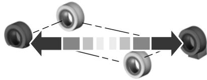
3. Block both the front and rear of the wheel diagonally opposite the flat tire. For example, if the left front tire is flat, block the right rear wheel.
