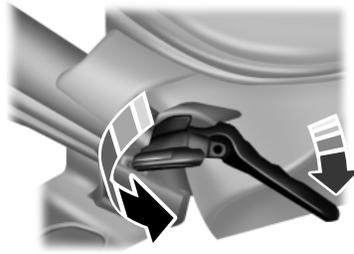
4. Pull down on the drivers latch handle and rotate it all the way forward into the windshield header.
