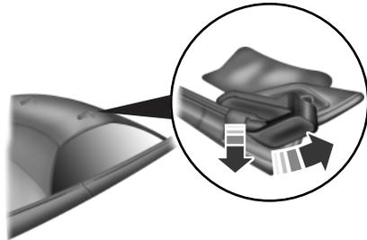
**Note:** The latch handles must be pulled downward fully to allow the latch to fully rotate into the open position.
