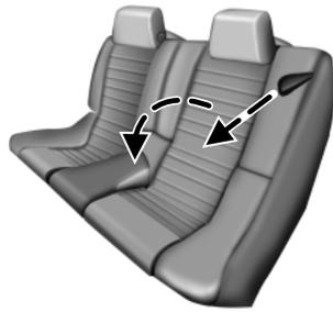
To lower the seat back(s) from inside the vehicle, be sure the head restraint is in the upright position, pull the strap to release the seat back and then fold the seat back down.
