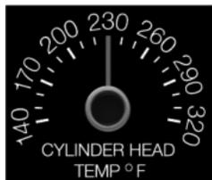
Displays the engine's cylinder head temperature.
