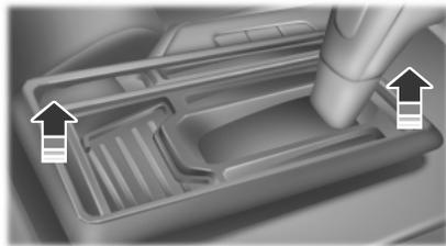
2. Using a flat head screwdriver or similar tool, remove the chrome bezel at the base of the gearshift lever.
