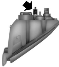
5. Then use a 7 mm Allen wrench or a Phillips screwdriver to adjust the vertical aim of the headlamp. HORIZONTAL AIM IS NOT REQUIRED FOR THIS VEHICLE AND IS NON-ADJUSTABLE.
