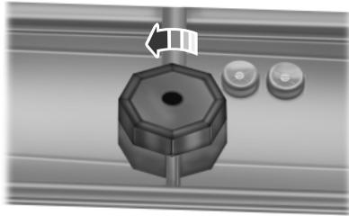
1. Clean the filler plug. It is located on the passenger side of the transmission.
