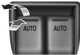
Press or lift the switches to operate the windows.
