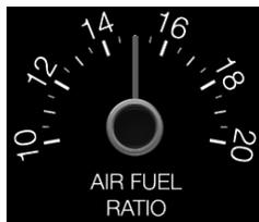
Displays the current air to fuel mixture in the engine.
