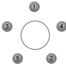
11. Remove the jack and fully tighten the lug nuts in the order shown. See *Wheel Lug Nut Torque Specifications* later in this chapter for the proper lug nut torque specification.
