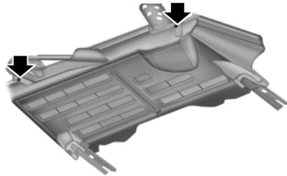
Some vehicles may be equipped with an aero-shield under the engine. Remove the front fasteners of the shield to gain access for service. This includes oil and filter changes.
