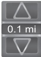
The map display scale has 17 levels, ranging from 0.02 miles (.03 kilometers) to 1000 miles (1600 kilometers). The system synchronizes the zoom scales for North Up, Heading Up and 3D Map views.
