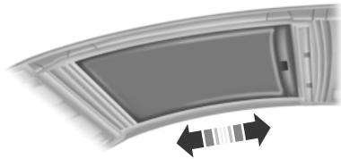
Use the center-mounted cup handle to slide the shade open or closed.
