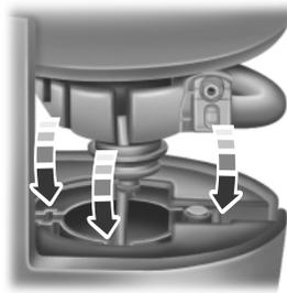
1. Align the sealant canister with the temporary mobility kit housing.
