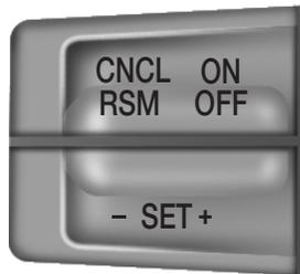
The cruise controls are located on the steering wheel.
