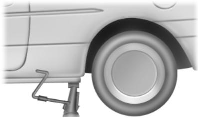
7. Put the jack in the jack notch next to the tire you are changing. Turn the jack handle clockwise until the wheel is completely off the ground.
