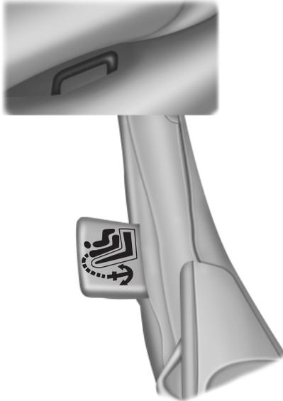
2. Access tether anchors located behind the seat back under the vinyl tag marked with the child tether anchor symbol.
