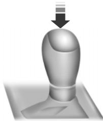
3. Shift into position R by pushing the gearshift knob down, then moving the lever fully to the left, then forward.
