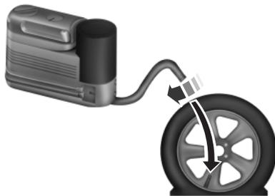
**Note:** When the sealing compound is first added into the tire, the air pressure gauge reading on the compressor unit may indicate a higher value; this is normal and should be no reason for concern. The pressure will drop after about 30 seconds of operation. The tire pressure has to be checked with the compressor in the OFF position to get the correct tire pressure reading.
