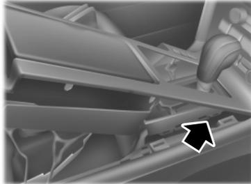
3. Lift the center console upward to access the base of the gear shifter assembly and locate the brakeshift interlock override lever.
