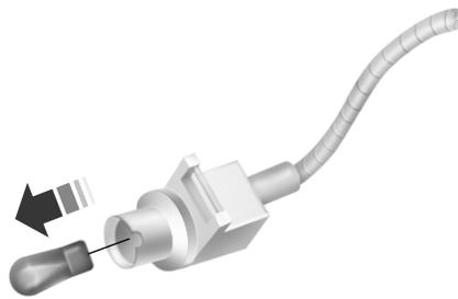
4. Carefully pull the bulb straight out of socket.
