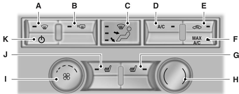
A. **Defrost:** Distributes air through the windshield defroster vents and demister vents. This setting can also be used to defog and clear the windshield of a thin covering of ice.
