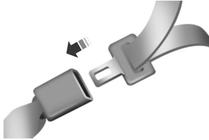
4. Insert the belt tongue into the proper buckle (the buckle closest to the direction the tongue is coming from) for that seating position until you hear a snap and feel the latch engage. Make sure the tongue is latched securely by pulling on it.
