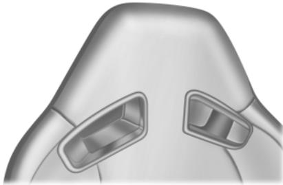
The non-adjustable head restraints consist of a trimmed foam covering over the upper structure of the seat back.
