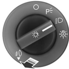
The fog lamps can be turned on when the lighting control is pulled toward you and in the headlamps, parking lamps or autolamps positions.
