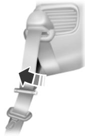
Rotate the presenter arm toward the front of the vehicle until it locks into place. This allows easier access to the front safety belt for the front seat occupant.
