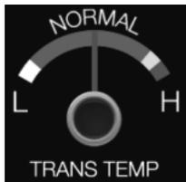
Displays the transmission fluid operating temperature. If the temperature rises to the red area, stop in a safe place and let the transmission cool. If the problem persists, see your authorized dealer.
