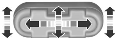
The power seat control is located on the outboard side of the seat. Move the switch in the direction of the arrows to raise or lower the seat cushion or to move the seat forward, backward, up or down.
