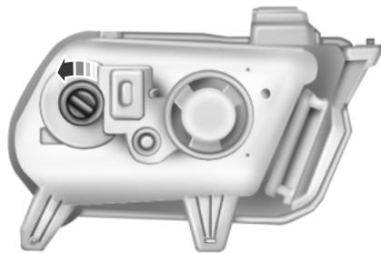
4. Rotate the socket counterclockwise and remove from the lamp assembly.
