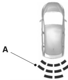
A. Coverage area of up to 6 feet (2 meters) from the rear bumper (with a decreased coverage area at the outer corners of the bumper).
