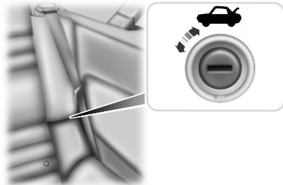
In the event of battery failure, you can open the trunk using your master key. The key cylinder is located between the rear seatback cushions on the driver's side.
