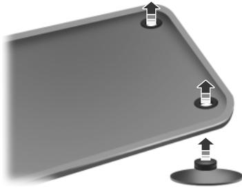
**!** **WARNING:** Always use floor mats that are designed to fit the foot well of your vehicle, leaving the pedal area unobstructed, and which can be firmly secured to retention posts so that they cannot slip out of position and interfere with the pedals or impair safe operation of your vehicle in other ways.
