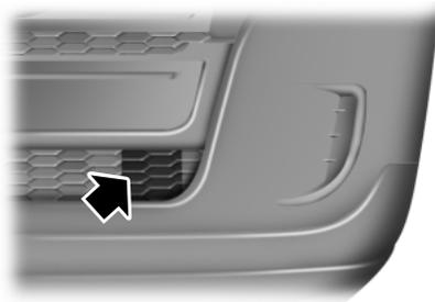
A message regarding a blocked sensor is displayed if the radar signals from the sensor have been obstructed. The sensor is located behind a fascia cover near the driver side of the lower grille. A vehicle ahead cannot be detected and the system will not function when the radar signals are obstructed. The following table lists possible causes and actions for this message being displayed.
