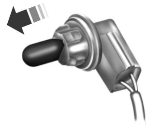
4. Pull bulb straight out of socket and push in the new bulb.
