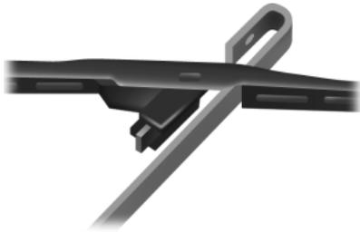
1. Pull the wiper arm away from the vehicle. Turn the blade at an angle from the wiper arm. Press the lock tab to release the blade and pull the wiper blade down toward the windshield to remove it from the arm.
