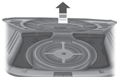
The system is located in the floor of the cargo area. Lift the release handle to open.
