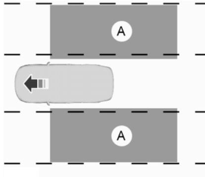
BLIS® aids the driver in detecting vehicles that may have entered the blind spot zone (A). The detection area is on both sides of the vehicle, extending rearward from the exterior mirrors to approximately 10 feet (3 meters) beyond the bumper. The system alerts you if certain vehicles enter the blind spot zone while driving.
