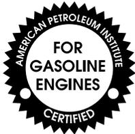
Only use oils certified for gasoline engines by the American Petroleum Institute (API). An oil with this trademark symbol conforms to the current engine and emission system protection standards and fuel economy requirements of the International Lubricants Specification Advisory Council (ILSAC), comprised of U.S. and Japanese automobile manufacturers.
