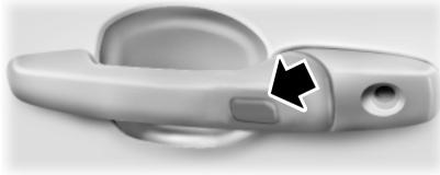
Press and hold the lock sensor area for about a second to lock your vehicle. To avoid unlocking the door inadvertently, make sure to only touch the lock sensor and not other areas of the door handle.
