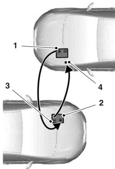
1. Connect the positive (+) jumper cable to the positive (+) terminal of the discharged battery.
