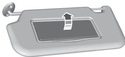
Lift the cover to switch on the lamp.
