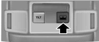
Pull and release the control. The moonroof will stop short of the fully closed position. Pull the control again and hold to fully close the moonroof.
