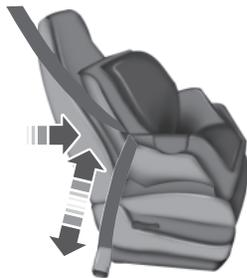
10. Before placing the child in the seat, forcibly move the seat forward and back to make sure the seat is securely held in place.
