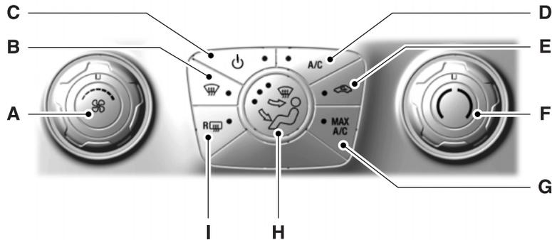
A. **Fan speed control:** Controls the volume of air circulated in your vehicle. Adjust to select the desired fan speed.
