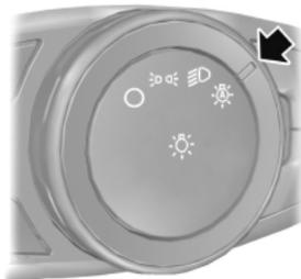
The autolamp system provides light sensitive automatic on-off control of the exterior lights normally controlled by the headlamp control.
