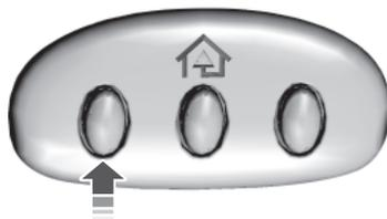
3. Using both hands, simultaneously press and hold the desired HomeLink button and the hand-held transmitter button. DO NOT release either one until the HomeLink indicator light flashes slowly and then rapidly. When the indicator light flashes rapidly, both buttons may be released. The rapid flashing indicates successful training.
