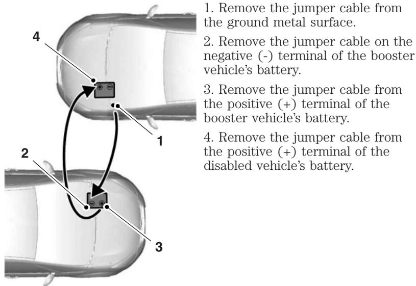
After the disabled vehicle has been started and the jumper cables removed, allow it to idle for several minutes so the engine computer can relearn its idle conditions.
