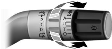
Use the rotary control to adjust the sensitivity to one of the interval moisture settings. The wipers will not cycle until moisture is detected on the windshield. The wiper speed will vary based on the amount of moisture detected on the windshield and the sensitivity setting.
