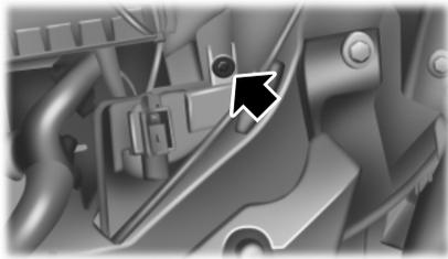
4. Locate the vertical adjuster on each headlamp. Using a Hex head driver, turn the adjuster either clockwise or counterclockwise in order to adjust the vertical aim of the headlamp.
