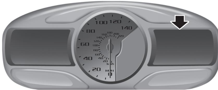
The display is located on the right side of your instrument cluster. You can use your steering wheel controls to view and make minor adjustments to active modes without taking your hands off the wheel. For example:
