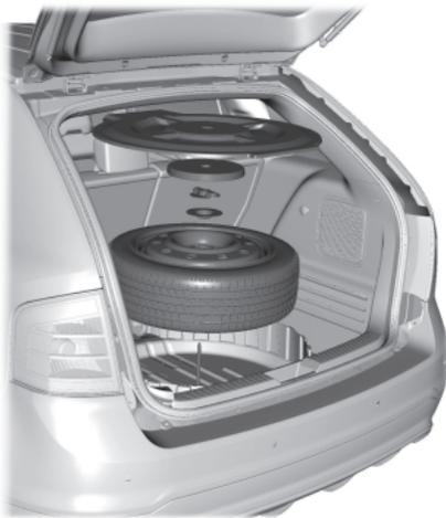
3. Lift the carpeted load floor panel located in the rear of the vehicle.
