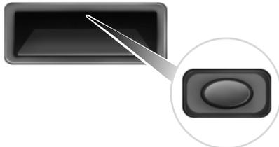
**To open the liftgate:** Press the button located in the top of the liftgate pull-cup handle to unlatch the liftgate, and then pull on the outside handle.
