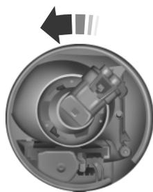
4. Turn the bulb holder counterclockwise and remove it.
