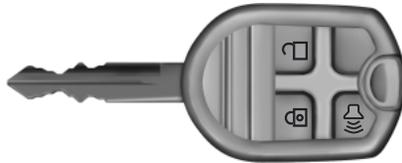
Use the key blade to start your vehicle and unlock or lock the driver door from outside your vehicle. The transmitter portion functions as the remote control.
