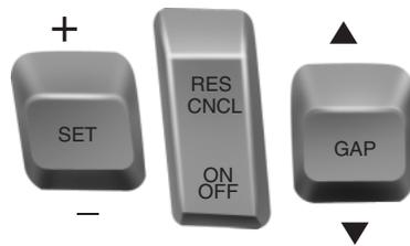
The controls for using your cruise control are located on the steering wheel.
