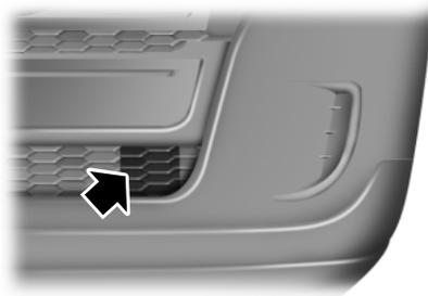
If a message regarding a blocked sensor appears in the information display, the radar signals from the sensor have been obstructed. The sensors are located behind a fascia cover near the driver side of the lower grille. When the sensors are obstructed, a vehicle ahead cannot be detected and the collision warning system does not function.
