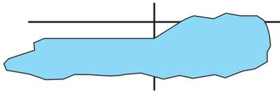
There is a distinct cut-off (change from light to dark) in the left portion of the beam pattern. The top edge of this cut-off should be positioned 2 inches (5 centimeters) below the horizontal reference line.
