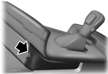
1. Using a screwdriver (or similar tool), carefully pry off and remove the BSI access panel.
