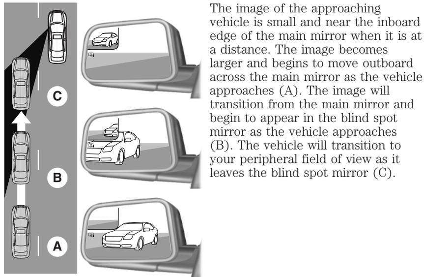
The image of the approaching vehicle is small and near the inboard edge of the main mirror when it is at a distance. The image becomes larger and begins to move outboard across the main mirror as the vehicle approaches (A). The image will transition from the main mirror and begin to appear in the blind spot mirror as the vehicle approaches (B). The vehicle will transition to your peripheral field of view as it leaves the blind spot mirror (C).
