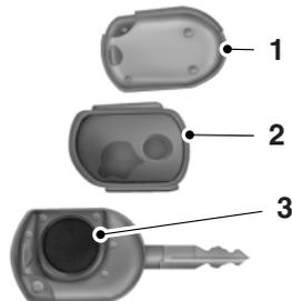
1. Twist a thin coin in the slot near the key ring to remove the battery cover (1).
