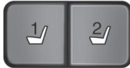
The memory control, located on the instrument panel, allows automatic positioning of the following features to two programmable positions:
