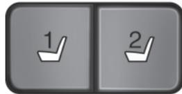
4. Press the lock button on the remote control within three seconds. Repeat this procedure with memory button **2** and a second transmitter if desired.
