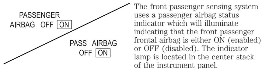
**Note:** When the ignition is first turned on, the passenger airbag status indicator OFF and ON lamps will illuminate for a short period of time to confirm it is functional.
