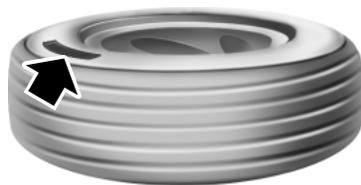
Tire Quality Grades apply to new pneumatic passenger car tires. The Tire Quality Grades can be found where applicable on the tire sidewall between tread shoulder and maximum section width. For example:
