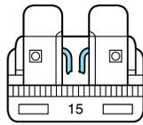
If electrical components in your vehicle are not working, a fuse may have blown. Blown fuses are identified by a broken wire within the fuse. Check the appropriate fuses before replacing any electrical components.
