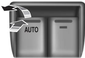
Press or lift the switches to operate the windows.
