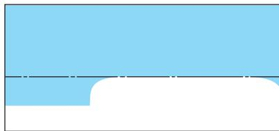
On the wall or screen you will observe a flat zone of high intensity light located at the top of the right hand portion of the beam pattern. If the top edge of the high intensity light zone is not at the horizontal reference line, the headlamp will need to be adjusted.
