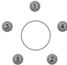
14. Remove the jack and fully tighten the lug nuts in the order shown. See *Wheel Lug Nut Torque Specifications* later in this chapter for the proper lug nut torque specification.
