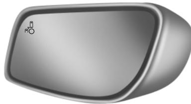
The BLIS® and CTA systems illuminate a yellow alert indicator in the outside mirror on the side of the vehicle the approaching vehicle is coming from.
