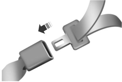
1. Insert the belt tongue into the proper buckle (the buckle closest to the direction the tongue is coming from) until you hear a snap and feel it latch. Make sure the tongue is securely fastened in the buckle.
