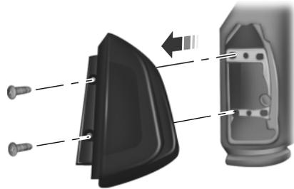
1. Make sure the headlamp switch is in the off position, then open the liftgate to expose the lamp assembly bolts.
