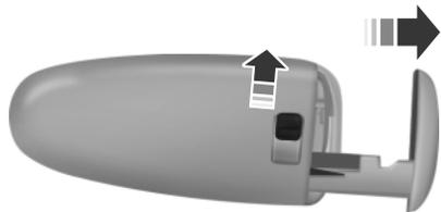
The intelligent access key also contains a removable mechanical key blade that you can use to unlock the driver door. Slide the release on the back of the transmitter to release the key blade, and then pull the blade out.
