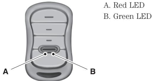
1. Press and hold one of the buttons on the hand-held transmitter for 10 seconds. The LED light will change from green to green and red.
