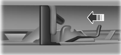
2. Go to the front of the vehicle and release the secondary hood latch that is located under the front center of the hood.
