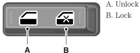
Press the control to lock or unlock the rear window controls.
