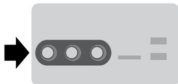
Your A/V inputs allow you to connect an auxiliary audio/video source (such as a gaming systems or a personal camcorder) by connecting RCA cords (not included) to these input jacks. The jacks are yellow, red and white and are located either behind a small access door on the
