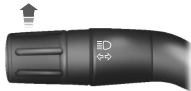
Push the lever forward to switch the high beams on.
