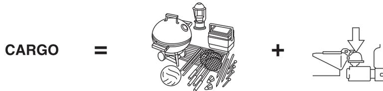
**Cargo Weight** – includes all weight added to the Base Curb Weight, including cargo and optional equipment. When towing, trailer tongue load weight is also part of cargo weight.
