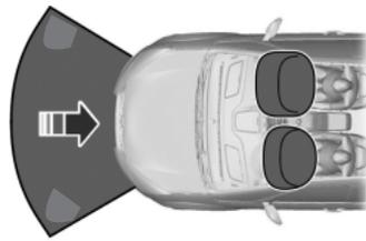
The driver and front passenger airbags will deploy during significant frontal and near-frontal crashes.
