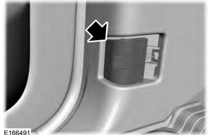
1. Inside the vehicle, pull the hood release handle located under the left hand side of the instrument panel.
