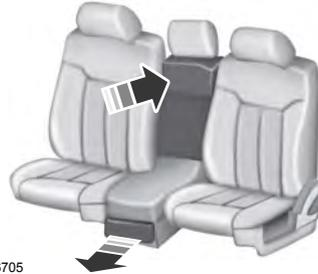
Press the release control to move the front seat armrest up or down.
