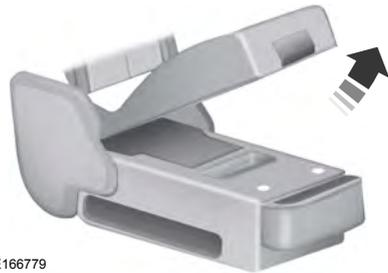
Lift the latch to open the lid and gain access to the optional storage compartment under the center seat cushion.
