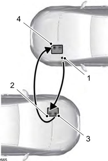
1. Remove the jumper cable from the ground metal surface or connecting point, if available.
