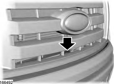
2. Go to the front of the vehicle and locate the secondary release lever. The release lever is located on the front bumper, under the grille.
