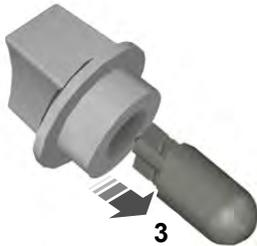
3. Remove the bulb by pulling it straight out.
