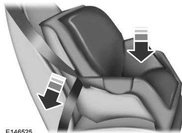
8. Remove remaining slack from the belt. Force the seat down with extra weight, for example, by pressing down or kneeling on the child restraint while pulling down on the lap belt in order to force slack from the belt. This is necessary to remove the remaining
