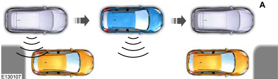
**Note:** If the direction indicators are not used, the system defaults to the passenger side of your vehicle.
