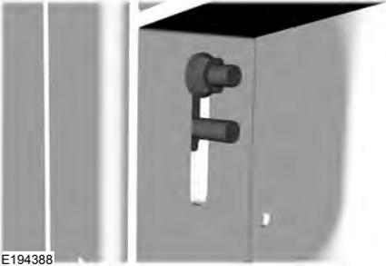
2. Slide the ramp holder studs upwards into the installed position.
