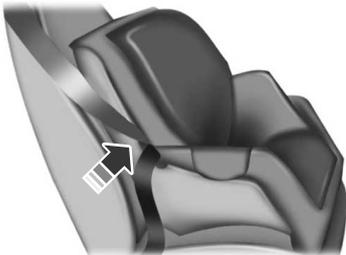
5. To put the retractor in the automatic locking mode, grasp the lap portion of the inflatable safety belt and pull upward until all of the belt is pulled out.
