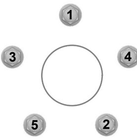
14. Remove the jack and fully tighten the lug nuts in the order shown. See **Changing a Road Wheel** (page 303).
