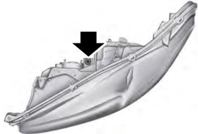
5. Locate the vertical adjuster on each headlamp. Using a Phillips #2 screwdriver, turn the adjuster either clockwise or counterclockwise in order to adjust the vertical aim of the headlamp. The horizontal edge of the brighter light should touch the horizontal reference line.
