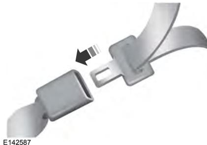
1. Insert the belt tongue into the proper buckle (the buckle closest to the direction the tongue is coming from) until you hear a snap and feel it latch. Make sure you securely fasten the tongue in the buckle.
