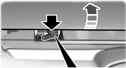
3. Lift the hood and support it with the prop rod.
