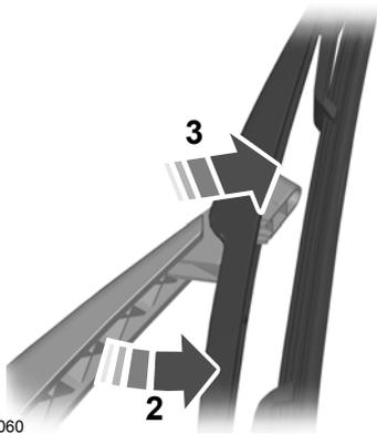
**Note:** Make sure that the wiper arm does not spring back against the glass when the wiper blade is not attached.
