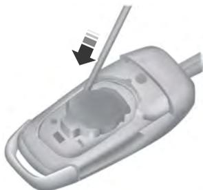
**Note:** Do not touch the battery contacts or the printed circuit board with the screwdriver.
