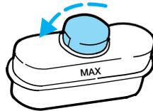
4. Use only a DOT 3 brake fluid certified to meet Ford specifications. Refer to *Lubricant specifications* in the *Capacities and specifications* chapter.
