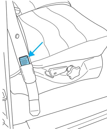
In the event of a collision, the colored label (REPLACE BELT) may become visible. If this occurs, *the safety belt must be replaced.*
