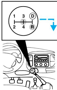
With the 6-speed transmission you can shift into R (Reverse) by moving the gearshift to the extreme left from N (Neutral).
