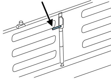
**Note:** When the vehicle is in motion, ensure the locking pins and knobs are fully engaged.
