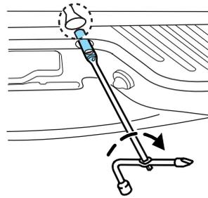
4. Turn the handle counterclockwise and lower the spare tire until you can slide the tire rearward and the cable is slack.
