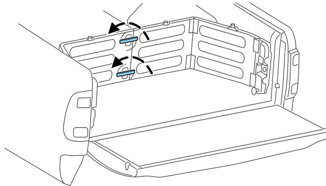
To open the bed extender into grocery mode, follow Steps 1–4 by rotating the panels away from the tailgate. Close the tailgate.
