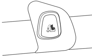
5. Clip the tether strap to the anchor as shown.
