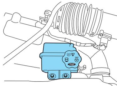
Check the fluid level when it is at ambient temperature, 20°F–80°F (-7°C–25°C):
