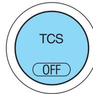
If you should become stuck in snow or ice or on a very slippery road surface, try switching the traction control system off. This may allow excess wheel spin to “dig” the vehicle out and enable a successful “rocking” maneuver.
