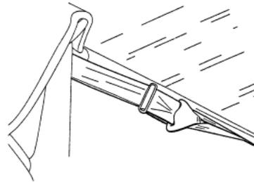
A single loop can be used to route and anchor more than one child seat. For example, the center loop can be used as a routing loop for a child safety seat in the center rear seat and as an anchoring loop for child seats installed in the outboard rear seats.
