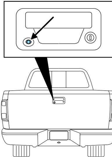
To use the camera system, place the transmission in R (Reverse); an image will display on the left portion of the rearview mirror or on the navigation screen (if equipped). The area displayed on the screen may vary according to the vehicle orientation and/or road condition.
