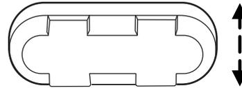
Press the control to move the seat forward, backward, up or down.
