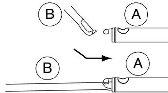
3. Fully insert the jack handle (with one extension) through the bumper hole and into the guide tube. The key and lock will engage with a slight push and counterclockwise turn. Some resistance will be felt when turning the jack handle assembly.
