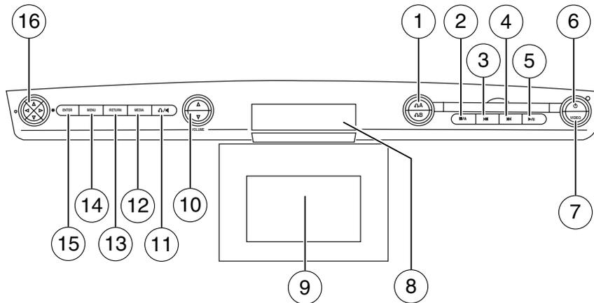
1. **Headphone control A/B:** While in Dual Play mode, press to select either the A or B headphone source. Then press MEDIA to select the desired playing media for that headset. When a headphone channel has been selected (A or B), selections will affect the source on that channel only.
