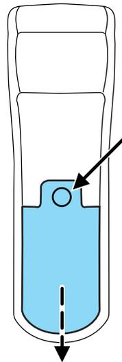
Remove the screw and unlatch the battery cover to access the batteries. The remote control unit uses two AAA batteries which are supplied with the unit.
