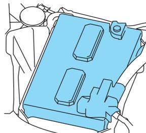
Your vehicle is equipped with a Motorcraft® maintenance-free battery which normally does not require additional water during its life of service.
