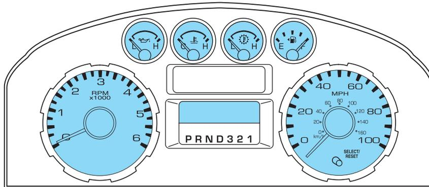
**Speedometer:** Indicates the current vehicle speed.
