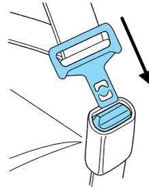
5. Put the safety belt in the automatic locking mode. To do so, grasp the shoulder portion of the belt and pull downward until all of the belt is pulled out.
