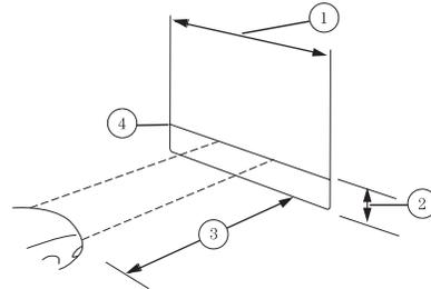
3. Turn on the low beam headlamps to illuminate the wall or screen and open the hood. Cover one of the headlamps so no light from that lamp hits the wall.
