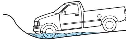
Once through water, always try the brakes. Wet brakes do not stop the vehicle as effectively as dry brakes. Drying can be improved by moving your vehicle slowly while applying light pressure on the brake pedal.
