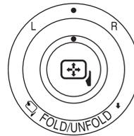
To operate the powerfold mirrors:
