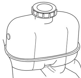
The fluid level will drop slowly as the brakes wear, and will rise when the brake components are replaced. Fluid levels between the MIN and MAX lines are within the normal operating range; there is no need to add fluid. If the fluid levels are outside of the normal operating range, the performance of your brake system could be compromised; seek service from your authorized dealer immediately.
