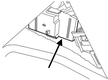
To remove a fuse use the fuse puller tool provided on the fuse panel cover.
