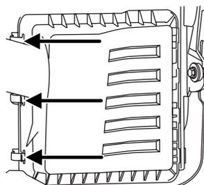
3. Pull air filter cover toward passenger side of vehicle and up to release the tabs. Lift air filter element up and out of housing.
