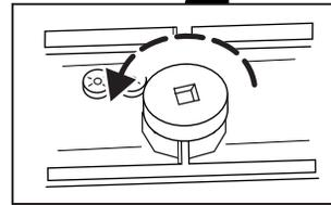
3. Fluid level should be at the bottom of the opening.
