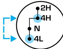
5. If shifting to 2H (2WD) with the vehicle at a complete stop, disengage the locking hubs (optional) by rotating the hub lock control from LOCK to FREE.
