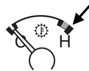
If the gauge is operating in the Yellow or Red area, stop the vehicle and verify the airflow is not restricted such as snow or debris blocking airflow through the grill. If the gauge continues to show high temperatures, see your authorized dealer.
