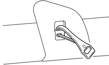
If the tether strap is clipped incorrectly, the child safety seat may not be retained properly in the event of a collision.
