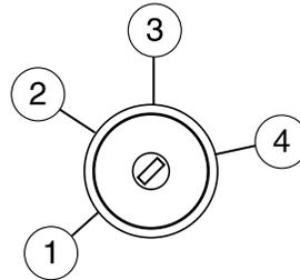
2. Turn ignition from the 3 (on) position back to the 1 (off) position in order to remove the first **coded key** from the ignition.
