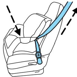
6. Attach the tether strap (if the child seat is equipped). Refer to *Attaching child safety seats with tether straps* later in this chapter.
