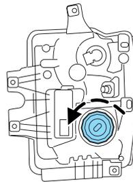
**!** **WARNING:** Handle a halogen headlamp bulb carefully and keep out of children's reach. Grasp the bulb only by its plastic base and do not touch the glass. The oil from your hand could cause the bulb to break the next time the headlamps are operated.
