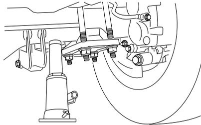
13. Insert the jack handle into the pump linkage.
