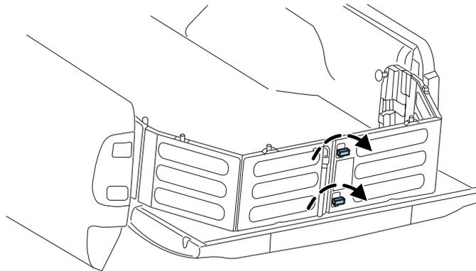
4. Connect the two panels, then rotate both knobs a quarter-turn clockwise to secure the panels.
