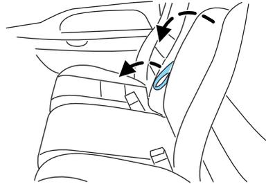
To gain access to the storage compartment in your armrest, lift the latch to open the lid. The lid cannot be opened in the upright position.
