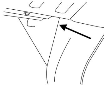
To remove the fuse panel cover, pull the panel toward you. When the clips of the panel disengage, let the panel fall easily.
