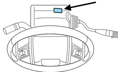
2. Apply the brake. Use a tool (or a small screwdriver) to pry out the access cover. Insert the tool into the access hole and slide the white override button towards the left. Move the gear shift lever into N (Neutral) while holding the white override disc towards the left.
