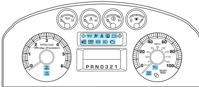
Warning lights and gauges can alert you to a vehicle condition that may become serious enough to cause expensive repairs. A warning light may illuminate when a problem exists with one of your vehicle's functions. Many lights will illuminate when you start your vehicle to make sure the
