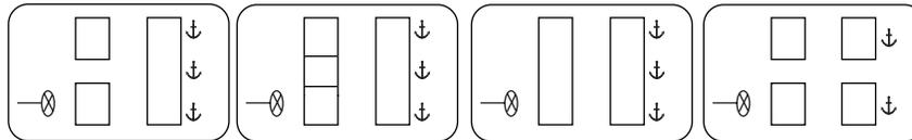
Attach the tether strap only to the appropriate tether anchor as shown. The tether strap may not work properly if attached somewhere other than the correct tether anchor.
