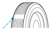
When replacing full size tires, never mix radial bias-belted, or bias-type tires. Use only the tire sizes that are listed on the Certification Label. Make sure that all tires are the same size, speed rating, and load-carrying capacity. Use only the tire combinations recommended on the label. If you do not follow these precautions, your vehicle may not drive properly and safely.
