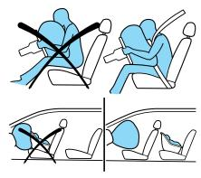
All occupants of the vehicle, including the driver, should always properly wear their safety belts, even when an air bag SRS is provided.
