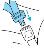
5. To put the retractor in the automatic locking mode, grasp the shoulder portion of the belt and pull downward until all of the belt is extracted
