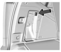
Insert an SD card into the card reader in the trunk. Disable the system from the playback screen before removing the SD card from the reader. Do not remove the card while recording is enabled. This could corrupt the video file and/or the SD card.
