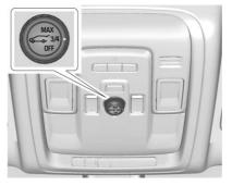
The power liftgate switch is on the overhead console. The vehicle must be in P (Park).
