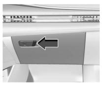
Pull the handle from the side to open the glove box. To close, push the glove box up until it latches. Use the mechanical key in the remote key to lock or unlock. See *Keys*  $\Rightarrow$  7.
