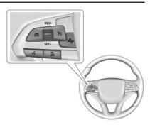
$\mathfrak{S}$ : Press to turn cruise control on or off. When ACC is the selected cruise control mode, the ACC indicator light  $\frown$  is lit white on the instrument cluster.
