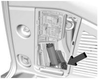
Turn the jack knob counterclockwise to release the jack and wheel blocks from the bracket. If equipped, remove the wheel blocks from the jack and place the wheel blocks on both sides of the tire at the opposite corner of the tire being changed. See If a Tire Goes Flat ⇒ 387 for more information on the placement of the wheel blocks. Place the jack and wheel blocks near the tire being changed.
