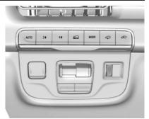
To activate each mode, press the MODE button on the instrument panel to the left of the steering wheel. To activate Terrain mode, press button located next to the MODE button.
