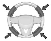
If your vehicle is equipped with Super Cruise or Lane Centering Assistance, hold the steering wheel in the indicated areas to help prevent unwanted take steering alerts.
