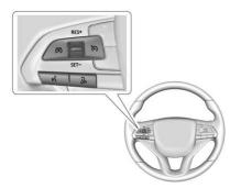
$\mathfrak{S}$ : Press to turn cruise control on or off. The cruise control indicator light  $\mathfrak{S}$  is lit white on the instrument cluster when cruise control is turned on.
