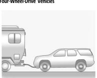
Only dinghy tow four-wheel-drive vehicles with a two speed transfer case that has an N (Neutral) and a 4 $\downarrow$  setting.
