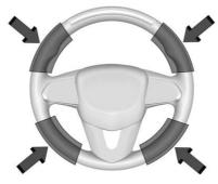
To begin steering manually, hold the steering wheel firmly with both hands using the highlighted regions. The Super Cruise indicator light will display red and a message will display in the DIC. In addition, beeps will sound, or the Safety Alert Seat will vibrate, if equipped. To view collision and detection settings from the infotainment home screen, touch Settings > Vehicle > Collision/Detection Systems. When you begin steering manually, Super Cruise will disengage.
