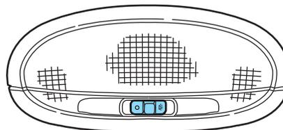
When the control is in the
