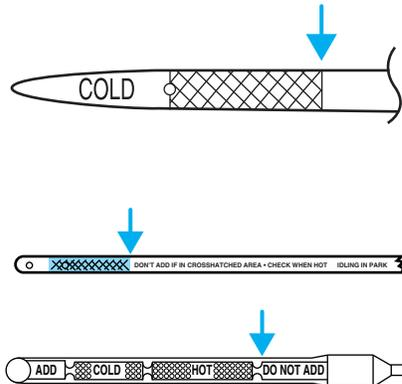
Fluid levels above the safe range may result in transmission failure.
