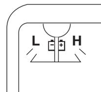
**Engine oil pressure gauge:** Indicates engine oil pressure. The needle should stay in the normal operating range (between "L" and "H"). If the needle falls below the normal range, stop the vehicle, turn off the engine and check the engine oil level. Add oil if needed. If the oil level is correct, have your vehicle checked by your authorized dealer.
