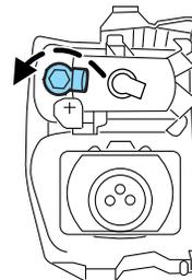
3. Rotate the bulb socket counterclockwise and remove.
