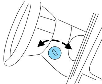
6. Cycle the ignition from off to on three (3) times ending in on. **DO NOT** start the engine.
