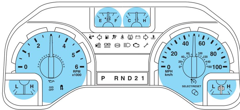
**Speedometer:** Indicates the current vehicle speed.
