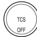
If you should become stuck in snow or ice or on a very slippery road surface, try switching the TCS off. This may allow excess wheel spin to “dig” the vehicle out and enable a successful “rocking” maneuver. Remember to switch the TCS back on once the vehicle is no longer stuck.
