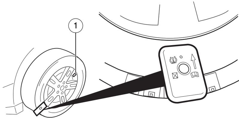
8. **Left front tire:** Place the TPMS reset tool against the left front tire where the tire meets the rim, opposite from the valve stem (1) as shown. This is where the sensor is located inside the rim.
