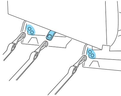
If the tether strap is clipped incorrectly, the child safety seat may not be retained properly in the event of a collision.
