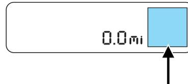
**Service engine soon:** The service engine soon indicator light illuminates when the ignition is first turned to the on position to check the bulb and to indicate whether the vehicle is ready for Inspection/Maintenance (I/M) testing. Normally, the "Service engine soon"
