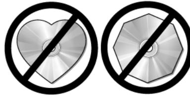
CDs with homemade paper (adhesive) labels should not be inserted into the CD player as the label may peel and cause the CD to become jammed. It is recommended that homemade CDs be identified with permanent felt tip marker rather than adhesive labels. Ballpoint pens may damage CDs. Please contact your authorized dealer for further information.
