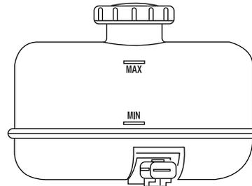
The fluid level will drop slowly as the brakes wear, and will rise when the brake components are replaced. Fluid levels between the MIN and MAX lines are within the normal operating range; there is no need to add fluid. If the fluid levels are outside of the normal operating range, the performance of the system could be compromised; seek service from your authorized dealer immediately.
