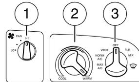
**MAX A/C:** Uses recirculated air to cool the vehicle. Air flows from the instrument panel vents only. If equipped with auxiliary A/C, auxiliary airflow will be from the rear headliner vents.
