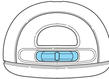
With the ignition key in the accessory or on position, the rear lamp can be turned on or off by sliding the control.
