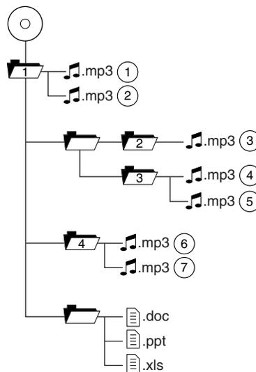
In track mode, the system will display and play the structure as if it were only one level deep (all .mp3 files will be played, regardless of being in a specific folder). In folder mode, the system will only play the .mp3 files in the current folder.
