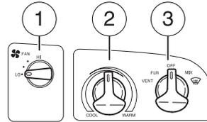
**VENT:** Distributes outside air through the instrument panel vents.
