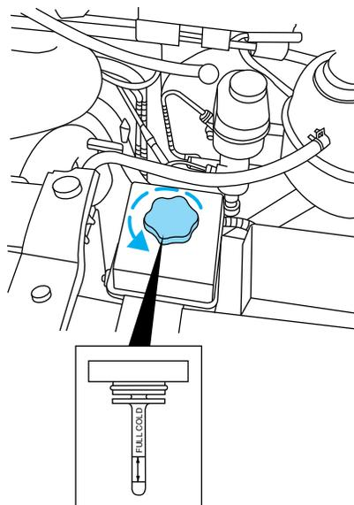
Check the fluid level when it is at ambient temperature, 20°-80°F
