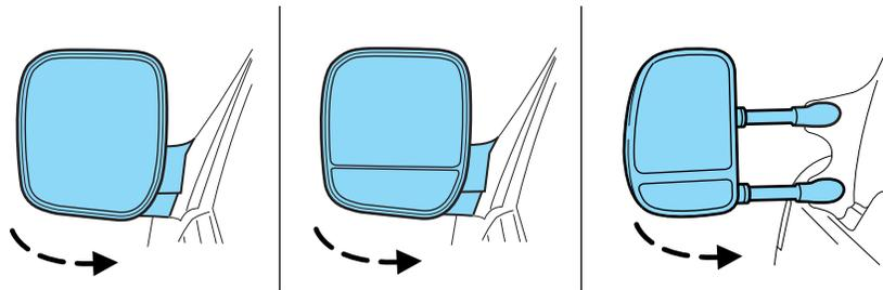
The telescoping feature (if equipped) allows the mirror to extend approximately 3.15 inches (80 mm). This feature is especially useful to the driver when towing a trailer.
