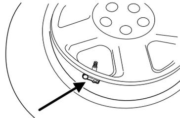
**Banded sensor — the pressure sensor is banded to the wheel.**
