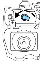
3. Rotate the bulb socket counterclockwise and remove.
