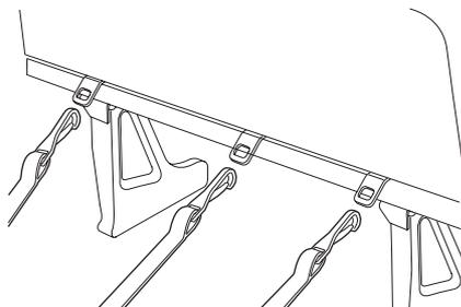
4. Refer to the instructions in this section under installing child safety seats in combination lap and shoulder belt seating positions to secure the child safety seat.
