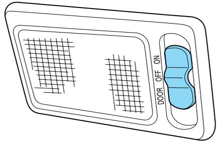
When the control is in the OFF position, it will not illuminate when you open the doors or fully rotate the headlamp control.
