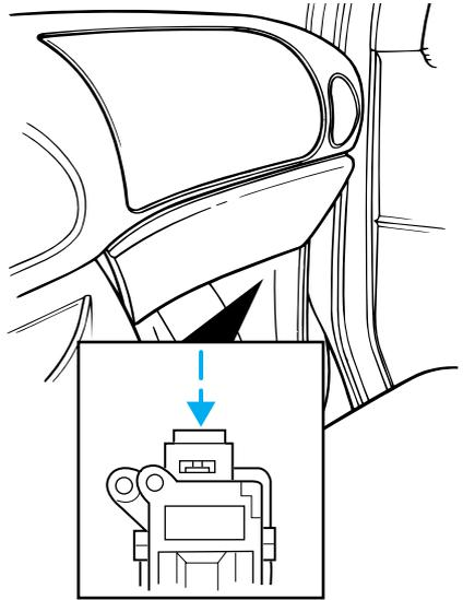
For commercial stripped chassis vehicles, the fuel pump shut-off switch is located on a bracket above the brake pedal.
