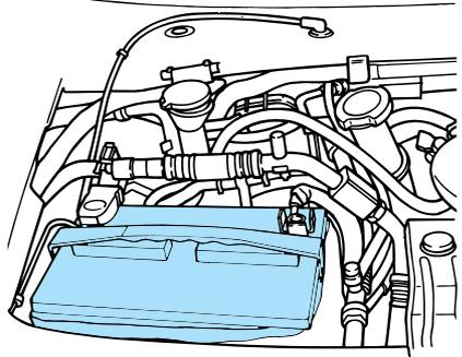
However, for severe usage or in high temperature climates, check the battery electrolyte level. Refer to the scheduled maintenance guide for the service interval schedules.
