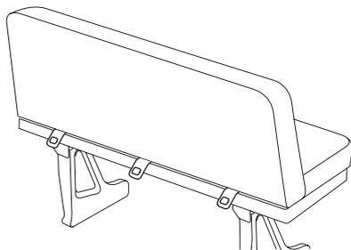
3. Clip the tether strap hook to the tether bracket mounted under rear rail of seat cushion frame as shown.
