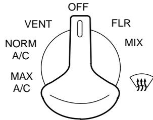
The air conditioning compressor can operate in all modes except VENT and FLR. However, the air conditioning will only function if the outside temperature is about 6°C (43°F) or higher.
