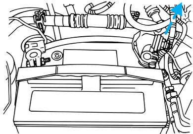
2. Wrap the secondary positive cable with a non-conductive material to insulate.
