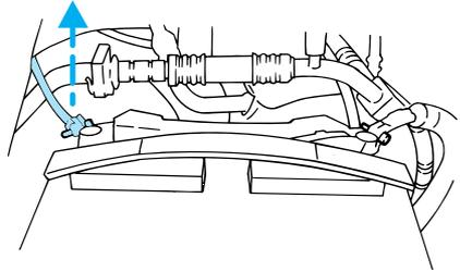
2. Disconnect the auxiliary battery frame ground.
