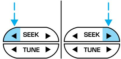
To set the minute, press and hold the CLK control and press TUNE:
