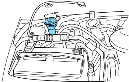
Only use a washer fluid that meets Ford specifications. Refer to *Lubricant specifications* in the *Capacities and specifications* chapter. State or local regulations on volatile organic compounds may restrict the use of methanol, a common windshield washer antifreeze additive. Washer fluids containing non-methanol antifreeze agents should be used only if they provide cold weather protection without damaging the vehicle's paint finish, wiper blades or washer system.
