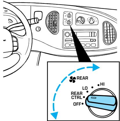
The fan speed of the auxiliary unit can be controlled either by the front seat using the front auxiliary control or by the rear seat passengers using the rear auxiliary control, but not both. To control the auxiliary unit using the rear control, the front control must be in the REAR position.
