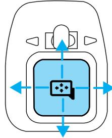
3. Return to the center position to lock mirrors in place.
