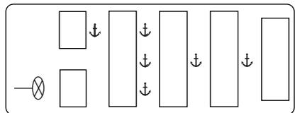
1. For second row 3-Passenger bench seat, place the child safety seat on the left hand outboard position, the center position, or the right hand outboard position as desired.
