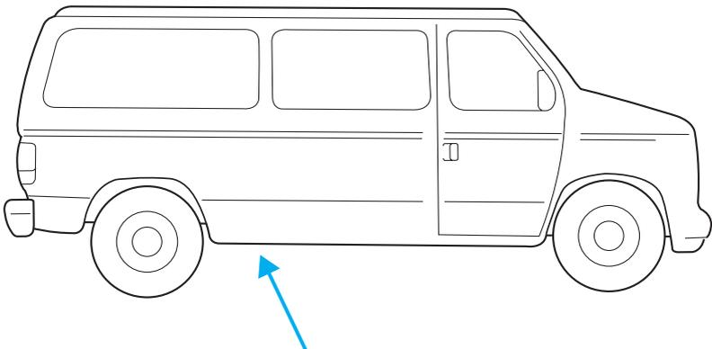
The auxiliary battery is located on the passenger side frame rail.
