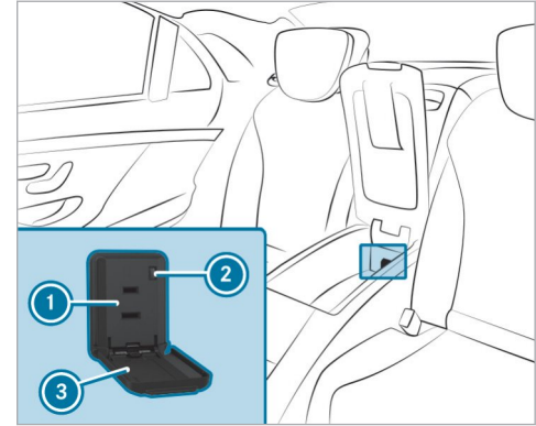
115 V socket in the center console of the rear passenger compartment (Mercedes-Maybach 4-seat vehicles)
