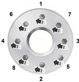
8-lug nut torque sequence
