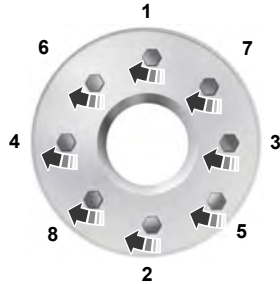
8-lug nut torque sequence
