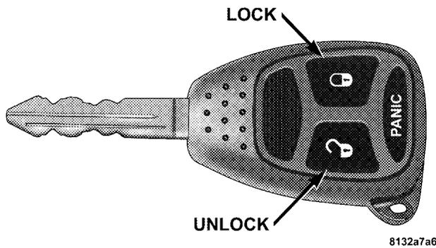
This system allows you to lock or unlock the doors and liftgate or activate the panic alarm from distances a minimum of 66 feet (20 meters) using a hand held radio transmitter. The transmitter need not be pointed at the vehicle to activate the system.
