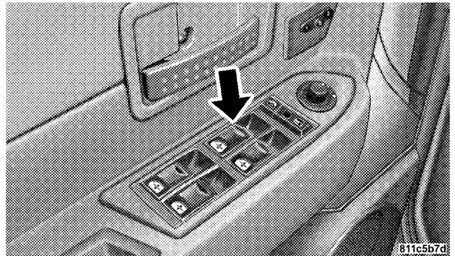
The control on the left front door has up-down switches that give you finger tip control of all four power windows. There is a single opening and closing switch on the passenger doors for passenger window control. The windows will operate only when the ignition switch is turned to the ON position and for ten minutes after the
