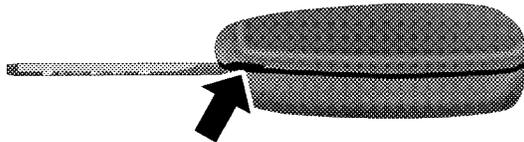
2. Remove and replace the batteries. Avoid touching the new batteries with your fingers. Skin oils may cause battery deterioration. If you touch a battery, clean it with rubbing alcohol.
