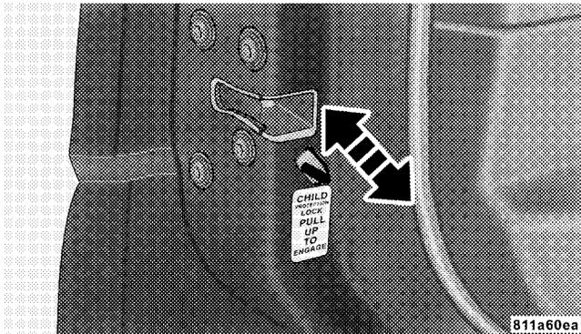
To use the system, open each rear door and slide the control UP to engage the locks and DOWN to disengage the child-protection locks. When the system on a door is engaged, that door can only be opened by using the outside door handle even if the inside door lock is in the unlocked position.
