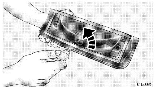
3. Pull bulb straight from socket to remove.
