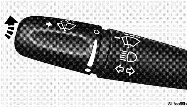
The wipers and washers are operated by a switch in the multifunction control lever. Turn the end of the handle to select the desired wiper speed.
