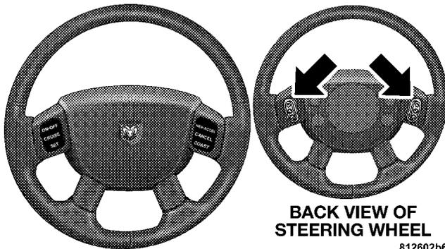
The right hand control is a rocker type switch with a push button in the center. Pressing the top of the switch will increase the volume and pressing the bottom of the switch will decrease the volume.
