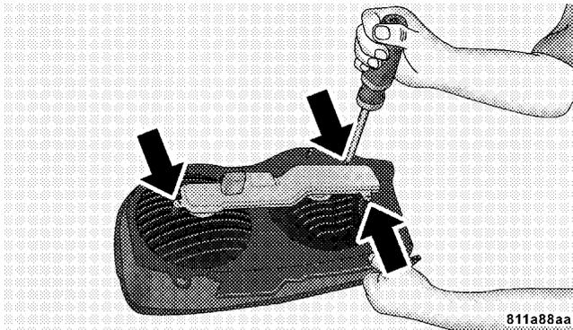
5. Remove the bulb strip from the tail light lens.
