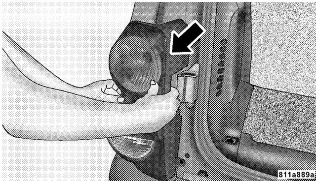
3. Unlock and remove electrical connector.
