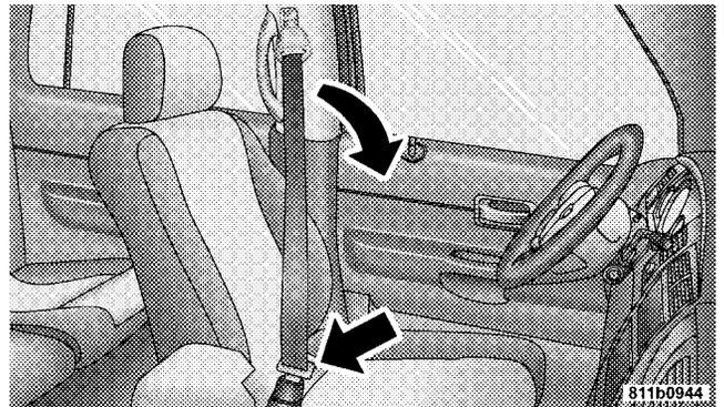
3. When the belt is long enough to fit, insert the latch plate into the buckle until you hear a “click.”
