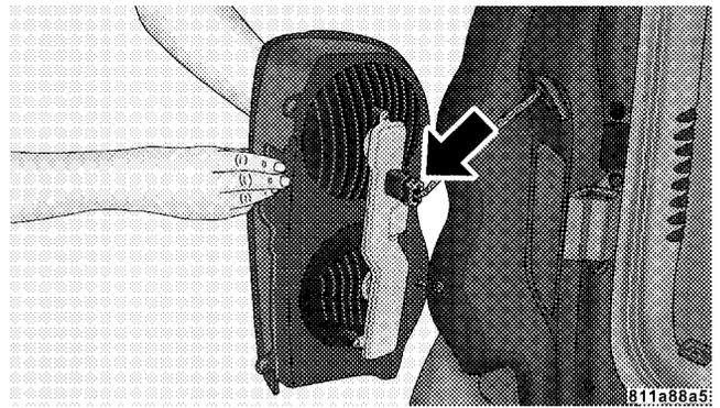
4. Remove the three screws holding the bulb strip to the back of the tail light lens.
