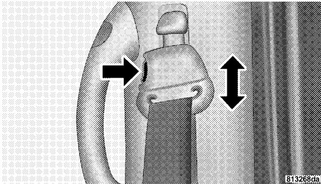
As a guide, if you are shorter than average, you will prefer a lower position, and if you are taller than average, you'll prefer a higher position. When you release the anchorage, try to move it up or down to make sure that it is locked in the desired position.
