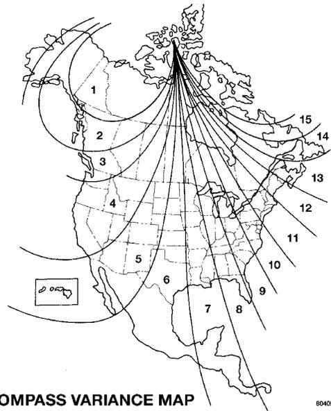
To set the variance: Turn the ignition ON and set the display to “Compass/Temperature.” Press and hold the RESET button approximately five seconds. The last variance zone number will be displayed. Press the STEP button to select the new variance zone and press the RESET button to resume normal operation.
