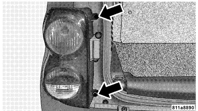
2. Rotate the light to the outboard side of the vehicle and remove.
