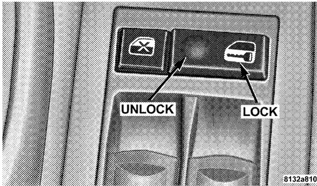
Vehicles equipped with power door locks can be locked or unlocked from inside by either the use of the door lock switches located on the front doors or by pressing the LOCK or UNLOCK buttons on the Remote Keyless Entry key fob.
