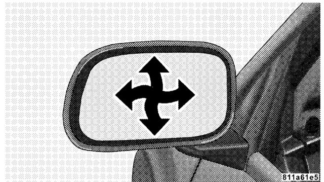
To adjust a mirror, turn the control wand toward the left or right mirror positions indicated. Tilt the control wand in the direction you want the mirror to move. When you are finished adjusting the mirror, turn the control to the center position to prevent accidentally moving a mirror.
