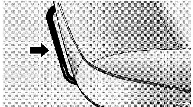
Using body pressure, move forward and rearward on the seat to be sure the seat adjusters have latched after the adjustment bar is released.
