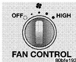
Use this control to regulate the amount of air forced through the system in any mode you select. Turn the control clockwise to increase fan speed. Turn the control to the full counterclockwise position to turn the fan off.
