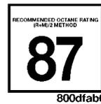
Your engine is designed to meet all emission regulations and provide excellent fuel economy and performance when using high quality unleaded “regular” gasoline having an octane rating of 87. The use of premium gasoline is not recommended.
