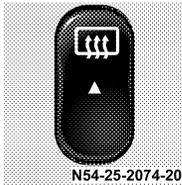
The switch for the heated rear window is located on the right-hand side next to the steering column.
