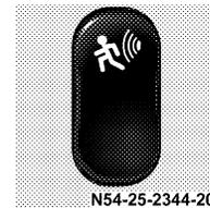
Trigger the alarm manually/lock the vehicle.
