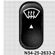
The switch for the windshield heater is located on the center section of the dashboard.
