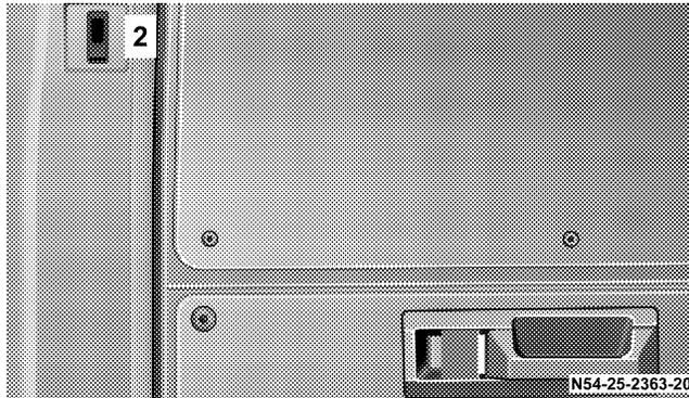
The switch (2) is located in the right rear of the cargo area.
