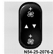
The auxiliary heat exchanger switch is located on the right next to the steering column.
