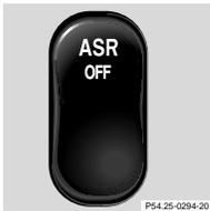
When driving with snow chains, in deep snow, or on sand or gravel, it can be beneficial to deactivate the acceleration skid control (ASR).
