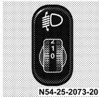
The range of the headlamps can be adjusted to the load in the vehicle.
