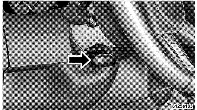
To unlock the steering column, pull the control handle outward. To tilt the steering column, move the steering wheel upward or downward as desired. To lengthen or shorten the steering column, pull the steering wheel outward or push it inward as desired. To lock the steering column in position, push the control handle inward until fully engaged.
