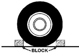
1. Block the wheel diagonally opposite the flat tire. Passengers should not remain in the vehicle when the vehicle is being jacked.
