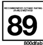
The 5.7L engine is designed to meet all emissions regulations and provide satisfactory fuel economy and performance when using high quality unleaded gasoline having an octane range of 87 to 89. The manufacturer recommends the use of 89 octane for optimum performance. The use of premium gasoline is not recommended. Under normal conditions, the use of
