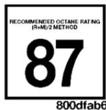
The 3.7L engine is designed to meet all emissions regulations and provide excellent fuel economy and performance when using high quality unleaded “regular” gasoline having an octane rating of 87. The use of premium gasoline is not recommended. Under normal conditions, the use of premium gasoline will not provide a benefit over high quality regular gasolines, and in some circumstances may result in poorer performance.
