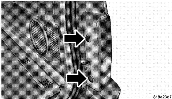
3. Pull lamp straight back and disconnect electrical connection.
