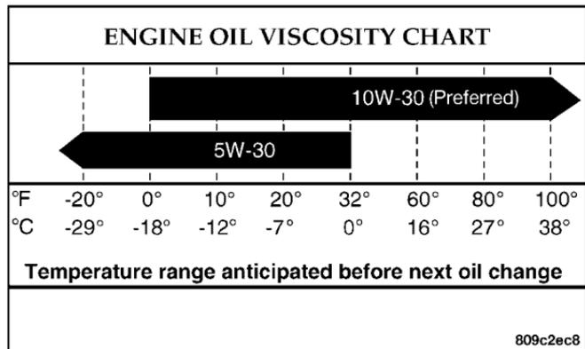
SAE **10W-30** engine oil is preferred. SAE **5W-30** engine oil is allowed during cold weather only to improve cold weather starting.
