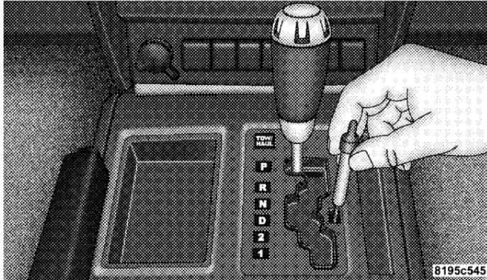
5. Move the shift lever into the N (Neutral) position.
