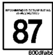
Your vehicle is designed to meet all emission regulations and provide excellent fuel economy when using high-quality regular unleaded gasoline with an octane rating of 87. The use of premium gasoline is not recommended, as it will not provide any benefit over regular gasoline in these engines.
