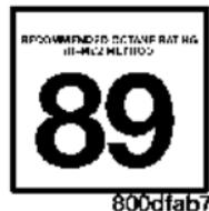
The 3.5L and 5.7L engines (with automatic transmission) are designed to meet all emissions regulations and provide satisfactory fuel economy and performance when using high-quality unleaded gasoline having an octane range of 87 to 89. The manufacturer recommends the use of 89 octane for optimum performance. The use of premium gasoline is not recommended, as it will not provide any benefit over regular gasoline in these engines.
