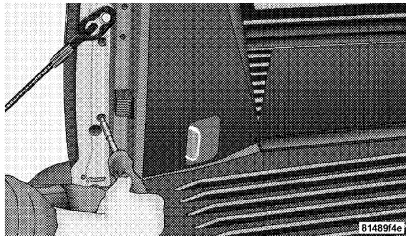
2. Pull the taillamp housing straight out from the body.
