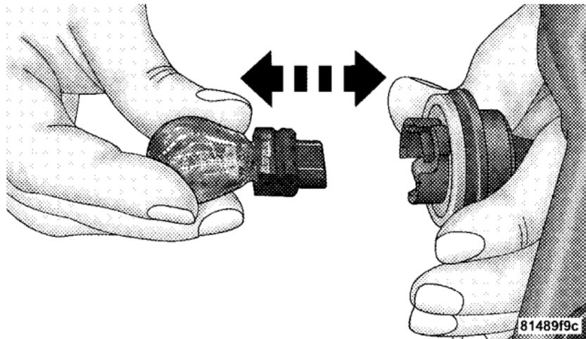
5. Reverse this procedure to install bulb and housing. Place the two raised blocks past the body.
