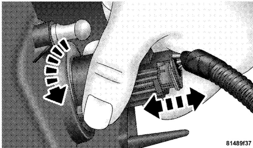
**NOTE:** The headlight bulb is a halogen bulb. Take care not to touch the bulb with your fingers. Body oils from your fingers could cause excessive heat buildup which reduces bulb life.
