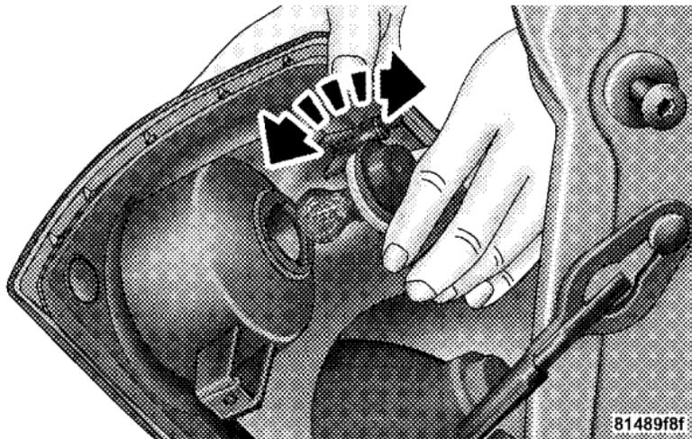
4. Pull bulb straight out of socket.
