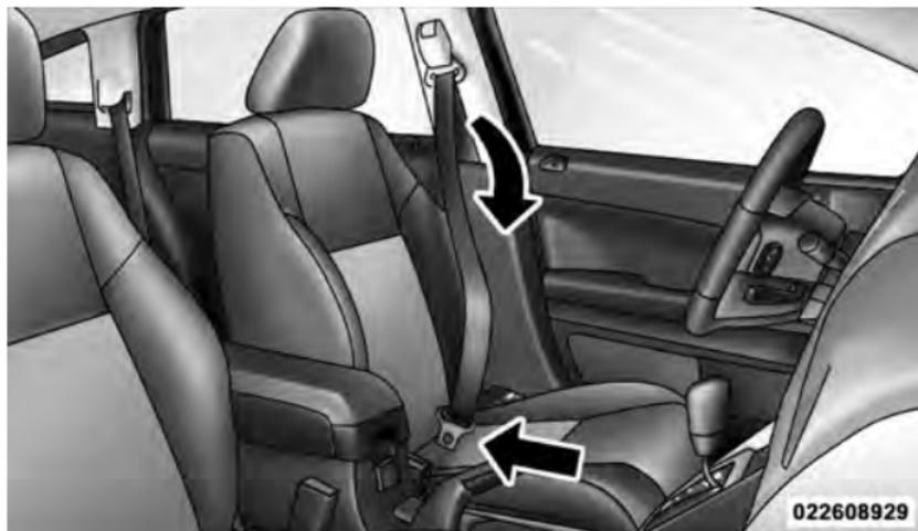
Inserting Latch Plate into Buckle
