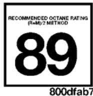
The 3.5L and 5.7L engine (with automatic transmission) is designed to meet all emissions regulations and provide satisfactory fuel economy and performance when using high-quality unleaded gasoline having an octane range of 87 to 89. The manufacturer recommends the use of 89 octane for optimum performance. The use of premium gasoline is not recommended, as it will not provide any benefit over regular gasoline in these engines.
