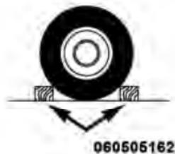
6. Block the front and rear of the wheel diagonally opposite of the jacking position. For example, if changing the right front tire, block the left rear wheel.
