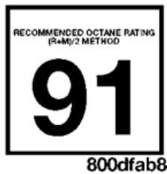
The 5.7L engine (with manual transmission) is designed to meet all emissions regulations and provide excellent fuel economy and performance when using high-quality premium unleaded gasoline with an octane rating of 91 or higher.
