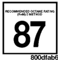
The 2.7L engine is designed to meet all emissions regulations and provide excellent fuel economy and performance when using high-quality unleaded “regular” gasoline having an octane rating of 87. The use of premium gasoline is not recommended, as it will not provide any benefit over regular gasoline in these engines.
