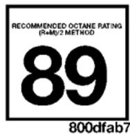
The 3.5L and 5.7L engine is designed to meet all emissions regulations and provide satisfactory fuel economy and performance when using high-quality unleaded gasoline having an octane range of 87 to 89. The manufacturer recommends the use of 89 octane for optimum performance. The use of
