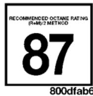
All engines are designed to meet all emissions regulations and provide excellent fuel economy and performance when using high quality unleaded “regular” gasoline having an octane rating of 87. The use of premium gasoline is not recommended, as it will not provide any benefit over regular gasoline in these engines.
