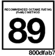
The 4.0L engine is designed to meet all emissions regulations and provide satisfactory fuel economy and performance when using high quality unleaded gasoline having an octane range of 87 to 89. The manufacturer recommends the use of 89 octane
