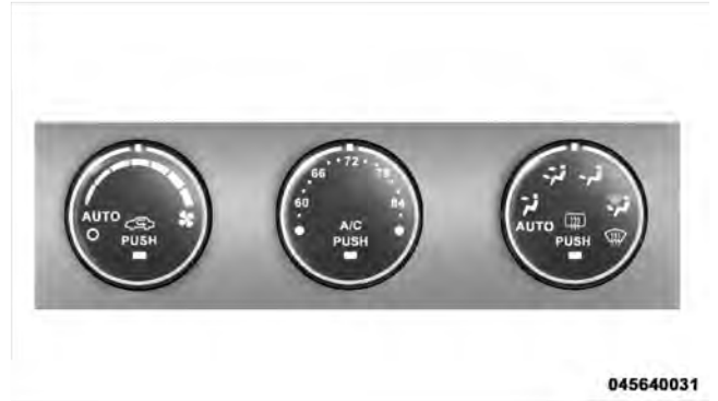
Automatic Temperature Control
