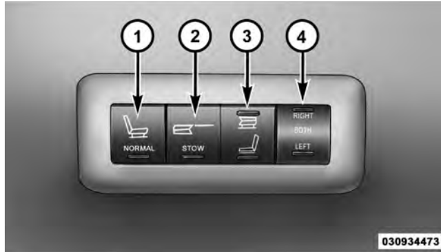
Rear Panel Power Switch Bank
