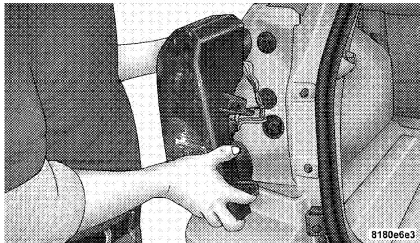
**NOTE:** It is not necessary to completely remove the tail lamp unit. Once loosened from the quarter panel, there should be enough room to service any of the bulbs.
