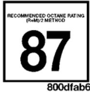
This engine is designed to meet all emissions regulations and provide excellent fuel economy and performance when using high-quality unleaded “regular” gasoline having an octane rating of 87. The use of premium gasoline is not recommended,
