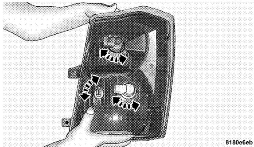
5. Remove the bulb from the socket and replace.
