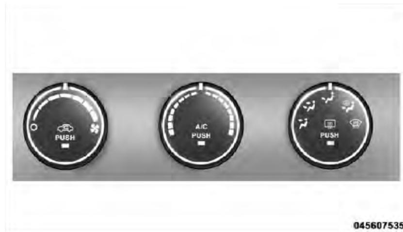
The Manual Temperature Controls consist of a series of outer rotary dials and inner push knobs.
